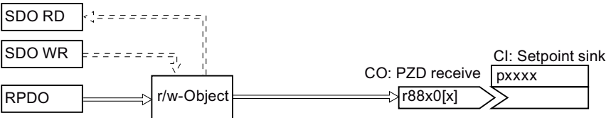
Figure 6-1 Access to mapped PZD setpoint objects
