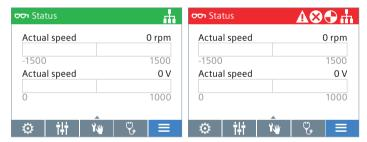
Figure 4-2 Fault and alarm notifications
