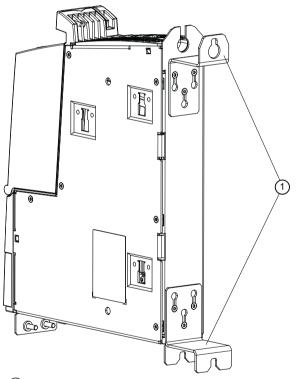
(1) Spacer Figure 4-17 CU320-2 with spacers for mounting on a mounting surface
