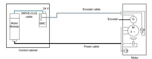
Figure 9-9 Connection of an encoder system via a Sensor Module Cabinet-Mounted (SMC) for a motor without a DRIVE-CLiQ interface
