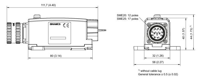
Figure 9-35 Dimension drawing of the Sensor Module External SME25, all data in mm and (inches)
