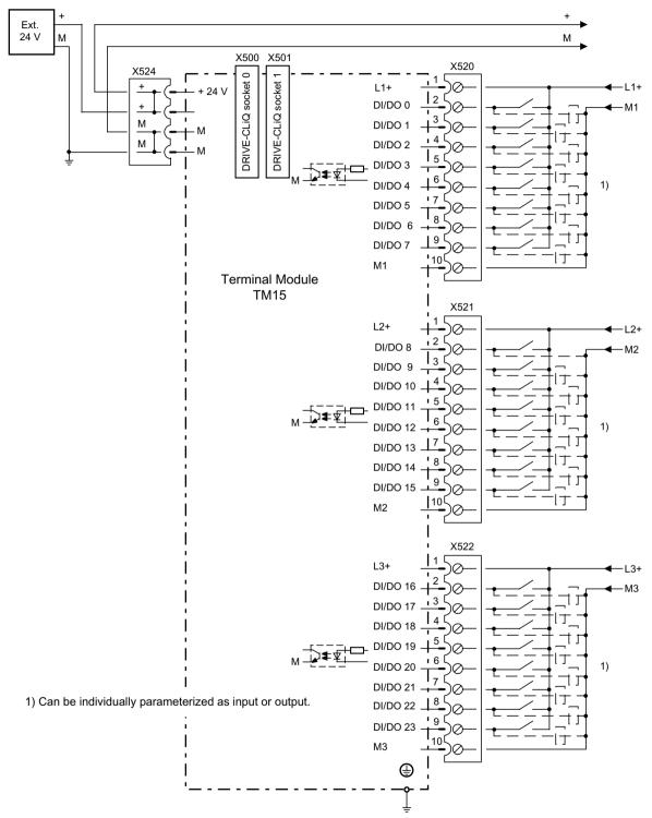
Figure 6-2 Example connection of TM15
