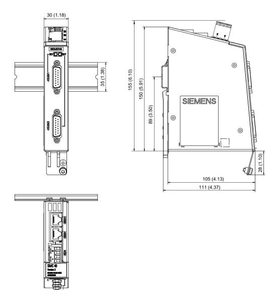
Figure 9-26 Dimension drawing of the Sensor Module Cabinet SMC40, all data in mm and (inches)
