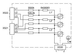
Figure 8-3 Internal circuit of the Voltage Sensing Module VSM10
