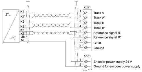
Figure 9-14 Connection example 1: HTL encoder, bipolar, with reference signal Signal cables must be twisted in pairs to improve immunity to induced noise.
