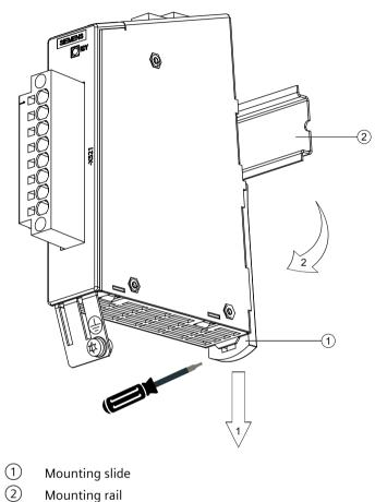
Figure 6-27 Removal of a TM120 from a DIN rail
