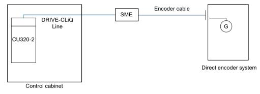
Figure 9-29 Connection of a direct encoder system via a Sensor Module External (SME)
