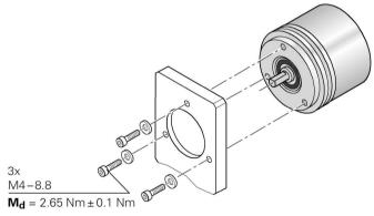
Figure 9-60 Installation: Synchro flange
