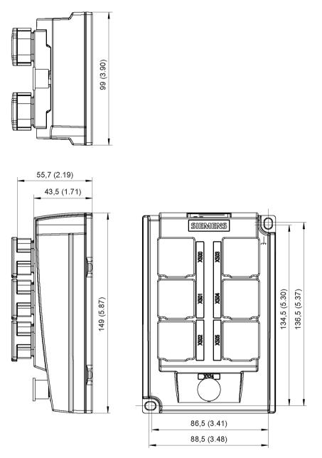
Figure 7-6 Dimension drawing of the DRIVE-CLiQ Hub Module External DME20, all data in mm and (inches)
