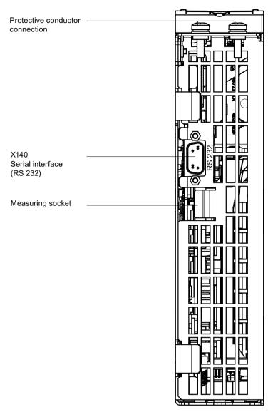
Figure 4-5 Interface X140 and measuring socket - CU320-2 PN (view from below)
