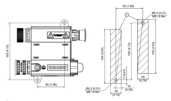
1 Contact surface Figure 9-45 Hole drilling pattern for installation
