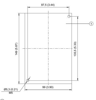
1 Contact surface Figure 7-7 Mounting dimensions DME20
