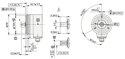
Figure 9-57 Dimension drawing of synchro flange, all data in mm
