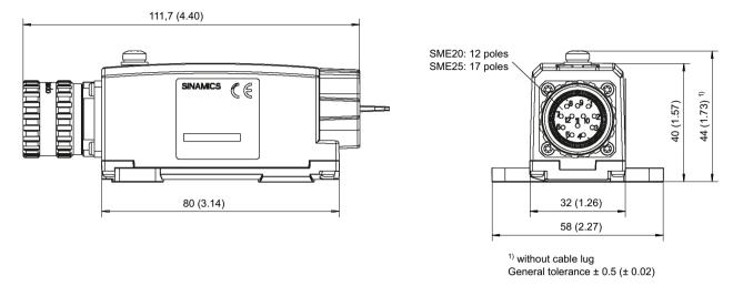
Figure 9-30 Dimension drawing of the Sensor Module External SME20, all data in mm and (inches)
