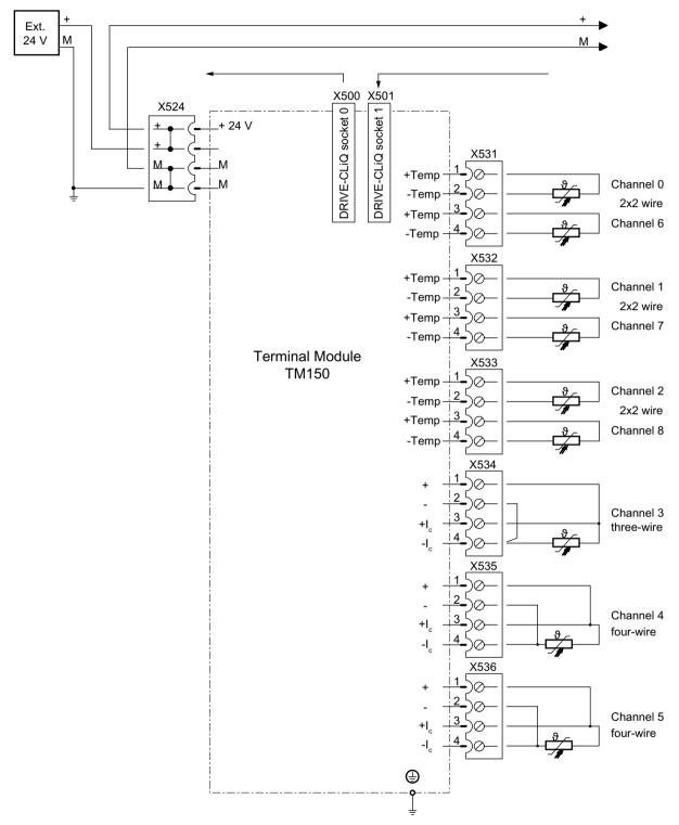
Figure 6-31 Connection example for a Terminal Module TM150
