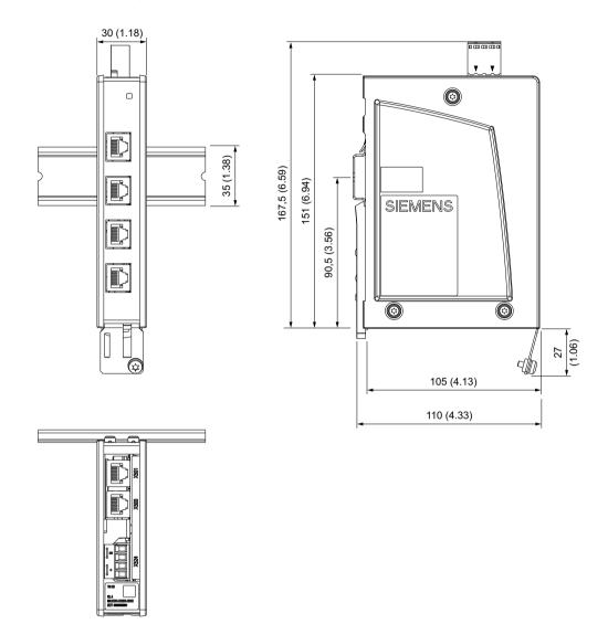
Figure 7-2 Dimension drawing of the DRIVE-CLiQ Hub Module DMC20, all data in mm and (inches)
