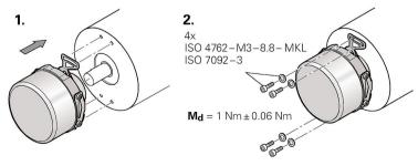
Figure 9-64 Installation: Hollow shaft
