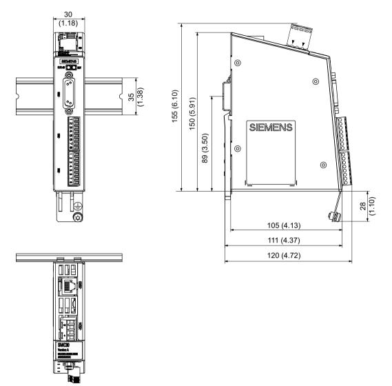
Figure 9-17 Dimension drawing of the Sensor Module Cabinet SMC30, all data in mm and (inches)
