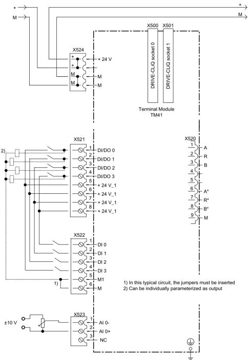
Figure 6-14 Sample connection of TM41
