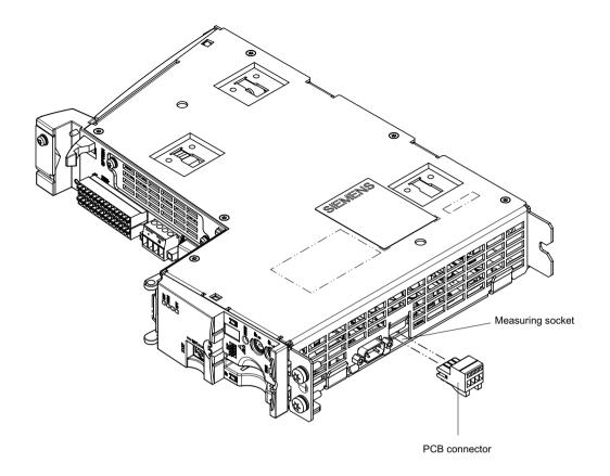
Figure 4-6 Mounting a PC board connector (Phoenix Contact) in the measuring socket
