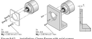
Figure 9-62 Installation: Clamp flange with axial screws
