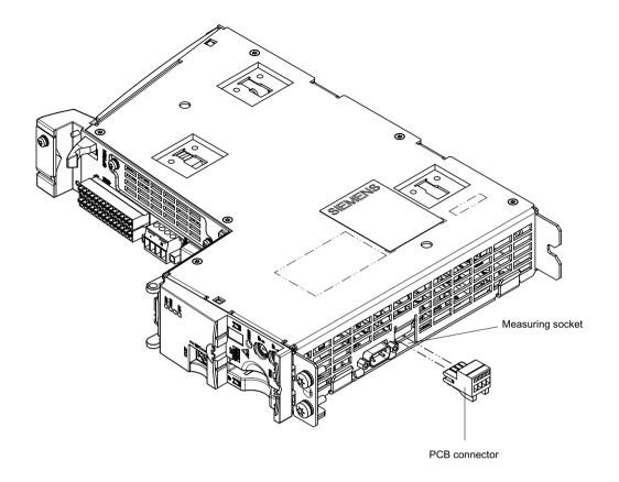
Figure 4-12 Mounting a PC board connector (Phoenix Contact) in the measuring socket
