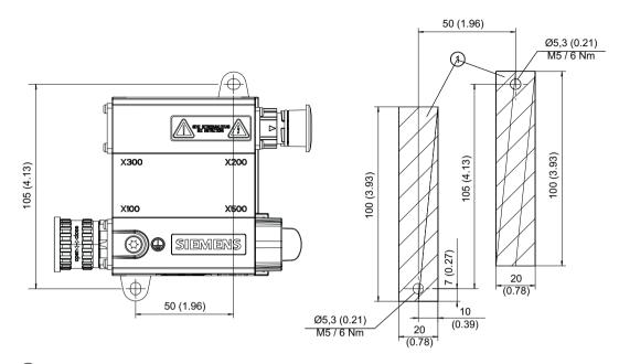
1 Contact surface Figure 9-54 Hole drilling pattern for installation
