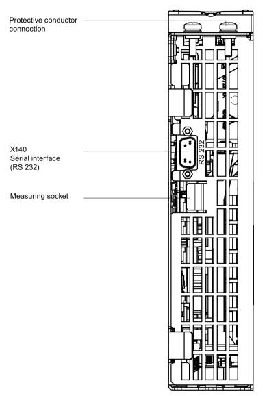
Figure 4-11 Interface X140 and measuring sockets T0 to T2 - CU320-2 DP (view from below)
