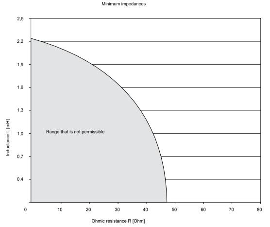
Figure 9-7 Rotor impedances that can be connected with excitation frequency f = 5000 Hz
