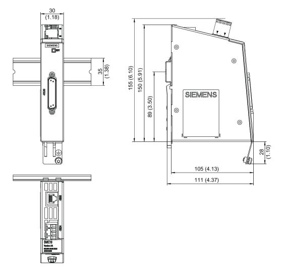
Figure 9-5 Dimension drawing of the Sensor Module Cabinet SMC10, all dimensions in mm and (inches)
