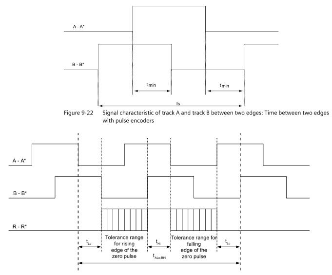
Figure 9-23 Position of the zero pulse to the track signals
