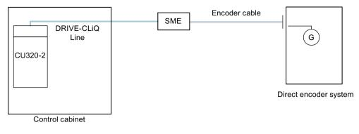
Figure 9-34 Connection of a direct encoder system via a Sensor Module External (SME)
