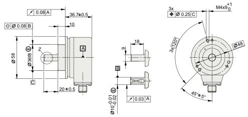
Figure 9-58 Dimension drawing of clamping flange, all data in mm
