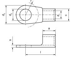
Figure 10-1 Dimension drawing of cable lugs
