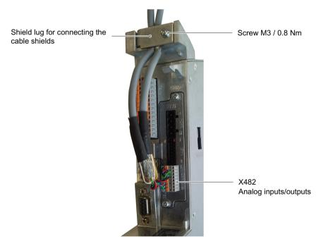
Figure 5-10 Shield support for TB30 on the CU320-2 DP
