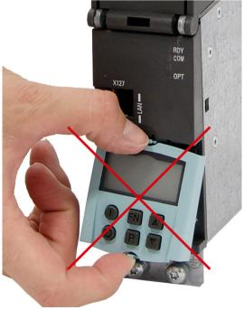
Figure 4-20 Incorrect removal of the BOP20 from a CU320-2 DP (example)
