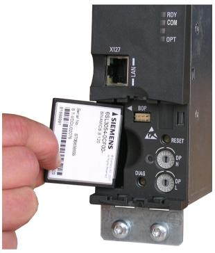
Figure 4-13 Slot for memory card
