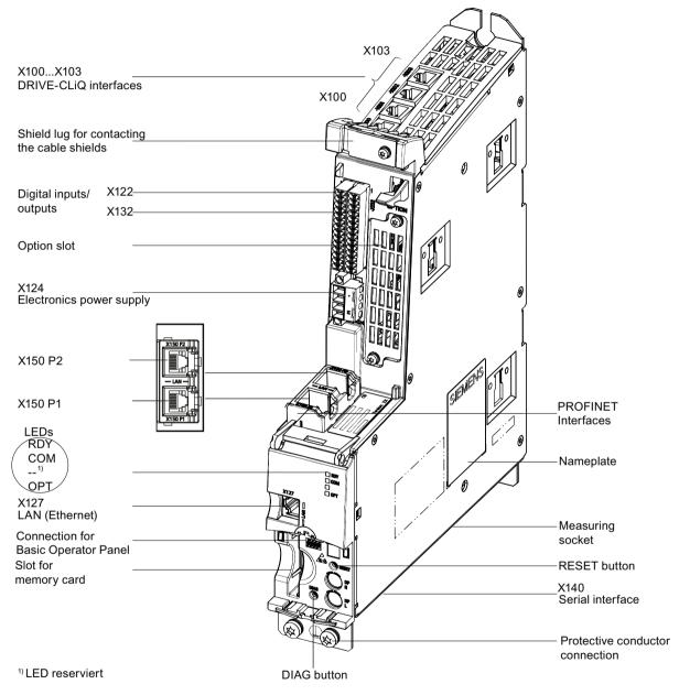
Figure 4-4 Interface overview CU320-2 PN (without cover and blanking cover)
