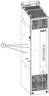
① Opening on the Line Module Chassis for fastening the Control Unit Figure 4-16 Mounting a Control Unit on a Line Module, chassis format 4.5 Mounting Control Units
