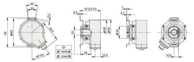
Figure 9-59 Dimension drawing of hollow shaft, all data in mm
