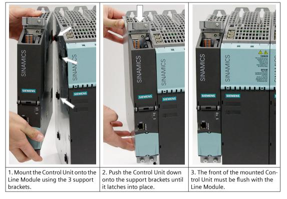
Table 4-32Installing the Control Unit on a Line Module using the CU320-2 DP as an example
