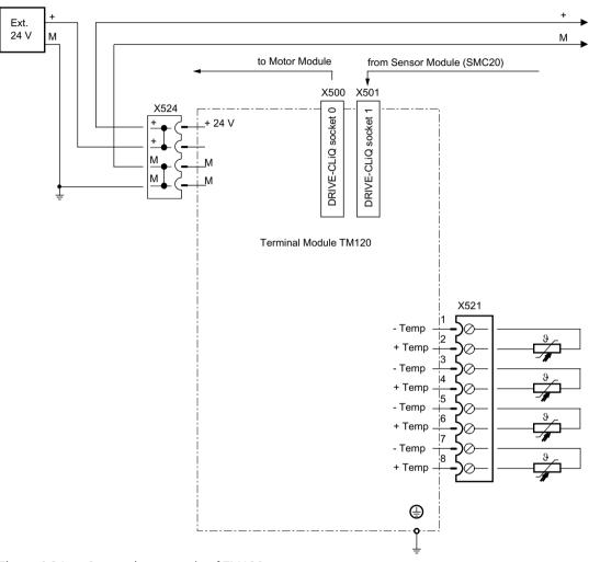
Figure 6-24 Connection example of TM120
