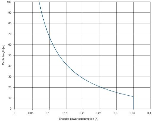
Figure 9-21 Max. cable length as a function of the encoder current drawn
