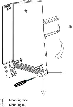
Figure 6-33 Removing a TM150 from a mounting rail
