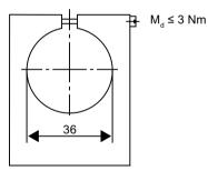
Figure 9-63 Installation: Clamp flange with slotted hole (not suitable for safety-related applications).
