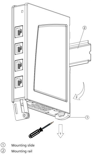
Figure 7-3 Removing from a DIN mounting rail
