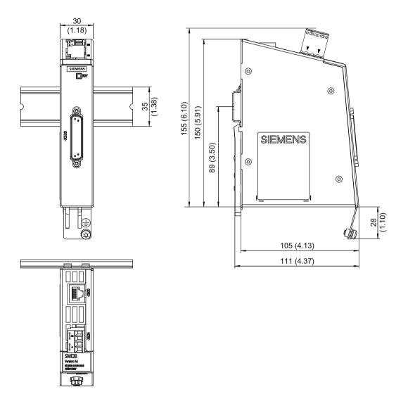
Figure 9-10 Dimension drawing of the Sensor Module Cabinet SMC20, all data in mm and (inches)
