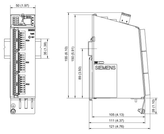
Figure 6-3 Dimension drawing of Terminal Module TM15, all data in mm and (inches)
