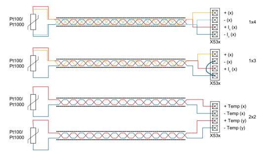
Figure 6-30 Connecting a Pt100/Pt1000 with 2x2, 3 and 4-wires to the temperature sensor inputs X53. of the TM150 Terminal Module
