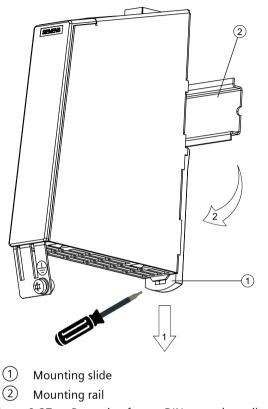
Figure 9-27 Removing from a DIN mounting rail
