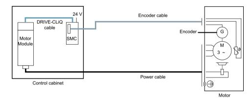
Figure 9-4 Connection of an encoder system via a Sensor Module Cabinet-Mounted (SMC) for a motor without a DRIVE-CLiQ interface
