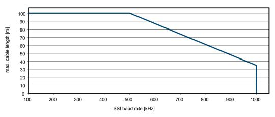
Figure 9-12 Maximum cable lengths depending on the SSI baud rate for SSI encoders
