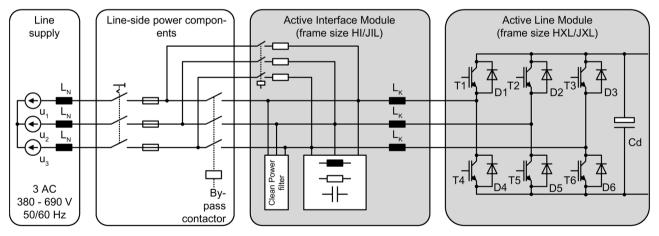
Figure 6-11 Overview of Active Infeeds, frame sizes HI/HXL and JI/JXL
