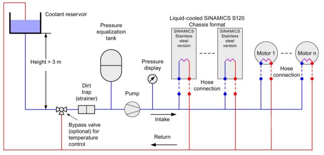
Figure 10-2 Recommendation for open circuit
