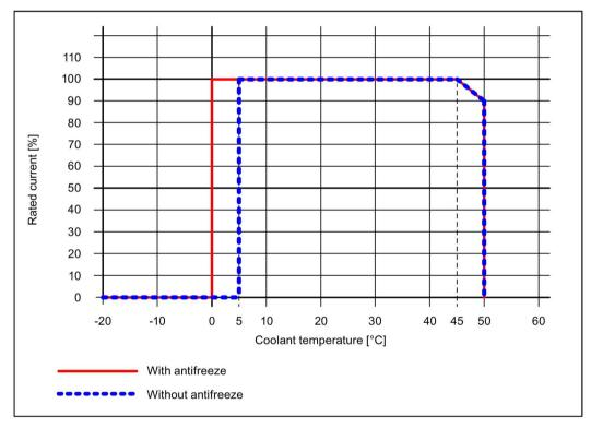
Figure 3-3 Maximum output current as a function of coolant temperature
