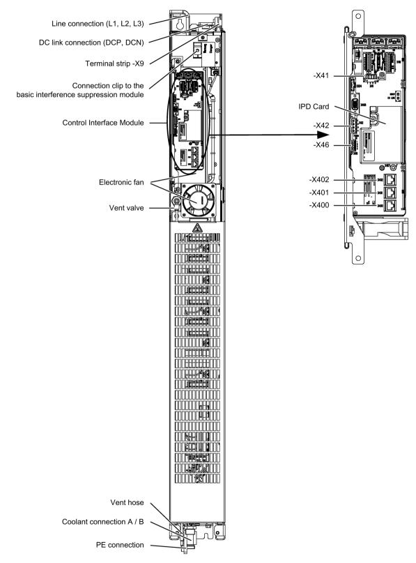
Figure 6-2 Basic Line Module, frame size GBL
