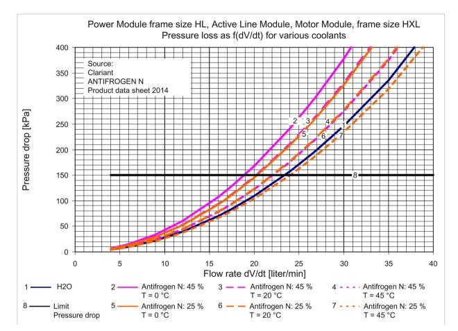
Figure 10-9 Pressure drop as a function of flow rate for Power Module frame size HL, Active Line Module and Motor Module frame size HXL
