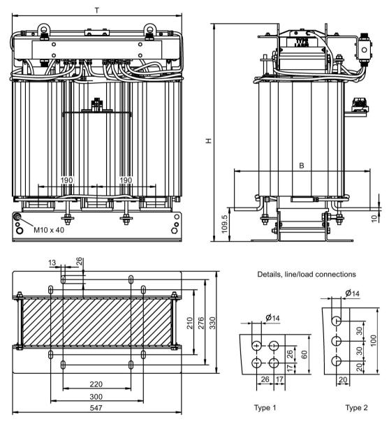
Figure 4-18 Dimension drawing, filter reactor frame size JIL
