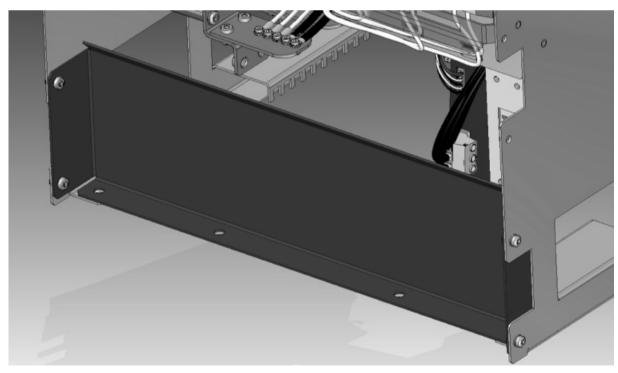
Figure 4-20 Transport plate on the underside of the filter module
