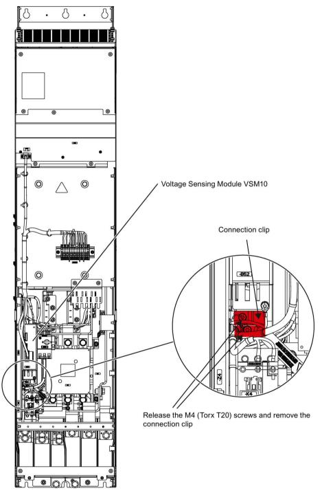
Figure 4-11 Removing the connection clip of the basic interference suppression module to ground for frame size GI
