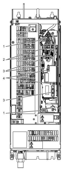
Figure 11-13 Replacing the electronic fan, Power Module, frame size FL
