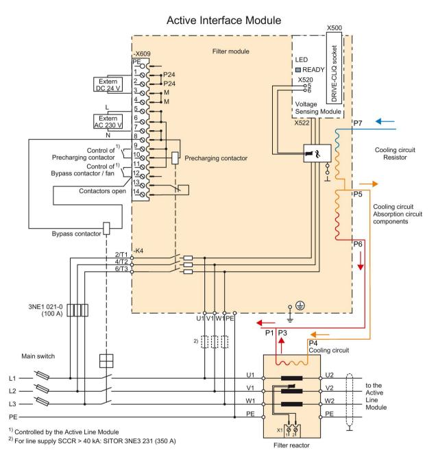
Figure 4-16 Connection example of liquid-cooled Active Interface Module, frame size JIL, valid for article numbers 6SL3305-7TE41-4AA5 and 6SL3305-7TG41-6AA5
