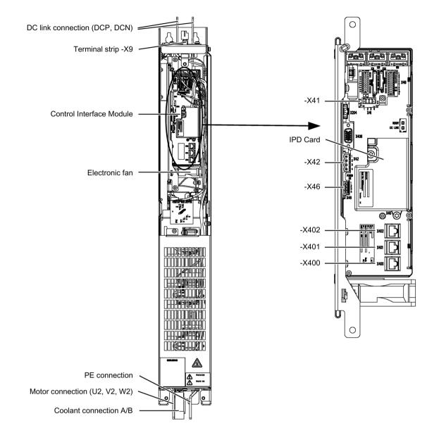
Figure 7-2 Motor Module, frame size GXL
