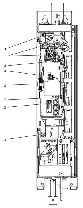
Figure 11-4 Replacing the Control Interface Module, Motor Module, frame size FXL
