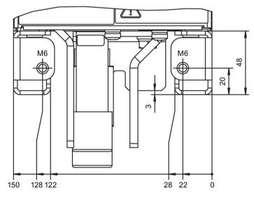
Figure 9-6 Rail profile, Active Line Module and Motor Module, frame size GXL, (dimensions in mm)
