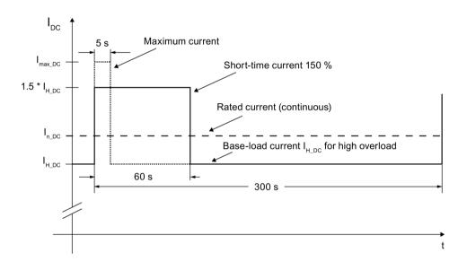
Figure 6-9 High overload
