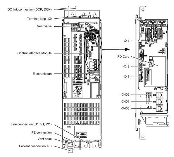
Figure 6-13 Active Line Module, frame size HXL
