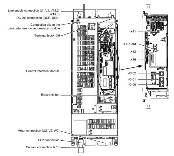
Figure 5-1 Power Module, frame size FL
