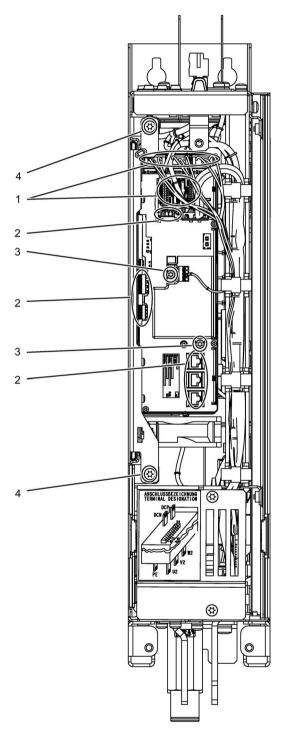
Figure 11-15 Replacing the electronic fan, Motor Module, frame size FXL
