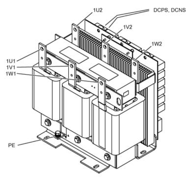
Figure 8-14 Interface overview for dv/dt filter compact plus Voltage Peak Limiter, Type 2
