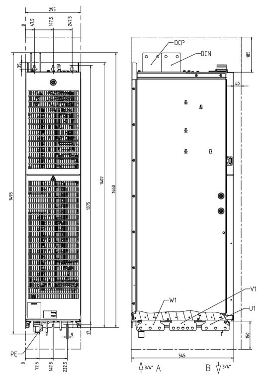
Figure 6-19 Dimension drawing Active Line Module, frame size JXL, article number 6SL3335-7TG41-6AA3. Front view, side view
