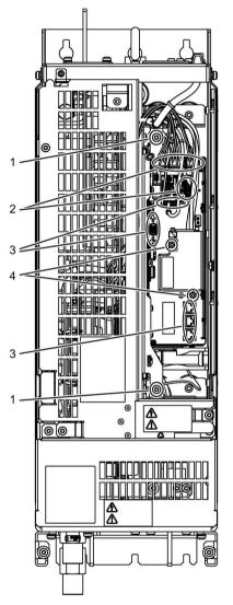
Figure 11-2 Replacing the Control Interface Module, Power Module, frame size FL
