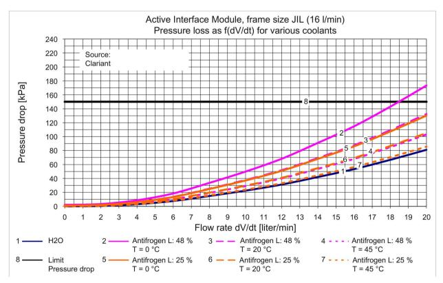
Figure 10-20 Pressure drop as a function of volumetric flow for Active Interface Module, frame size JIL, 16 l/min
