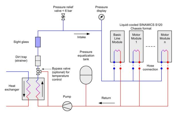
Figure 10-1 Recommendation for closed circuit
