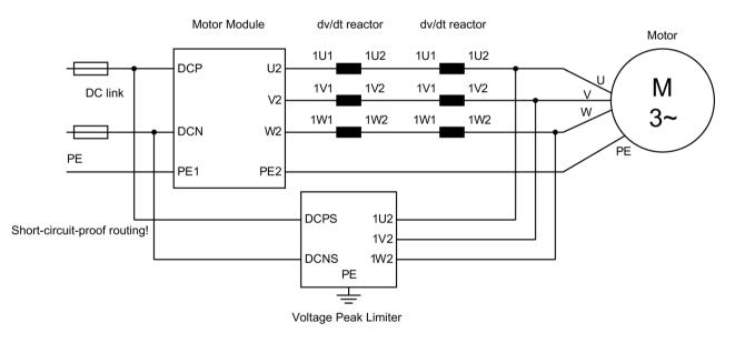
Figure 8-8 Connecting a dv/dt filter plus voltage peak limiter for versions with two dv/dt reactors
