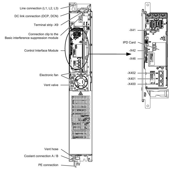
Figure 6-1 Basic Line Module, frame size FBL
