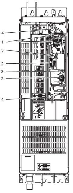
Figure 11-17 Replacing the electronic fan, Active Line Module, and Motor Module, frame size HXL
