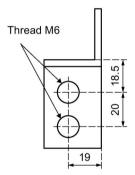
Figure 9-2 Bolting points for the mounting rails (dimensions in mm)
