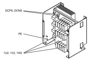
Figure 8-4 Interface overview, voltage peak limiter, type 1
