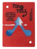
Figure 2-3 Tilt indicator tripped
