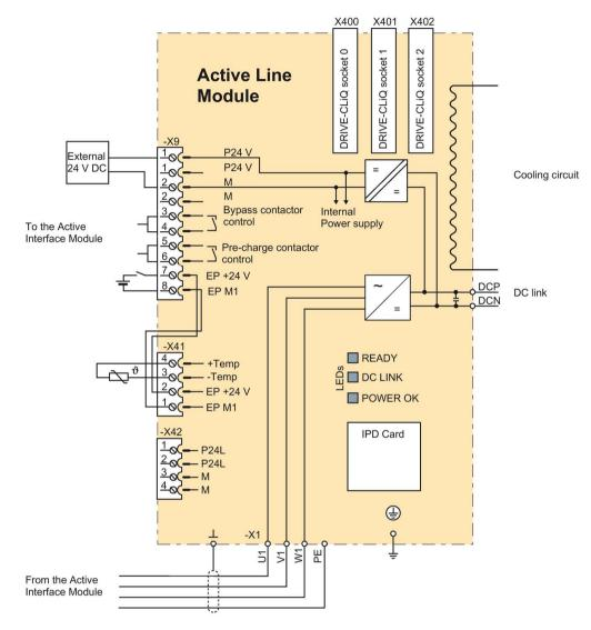
Figure 6-15 Example connection of Active Line Module
