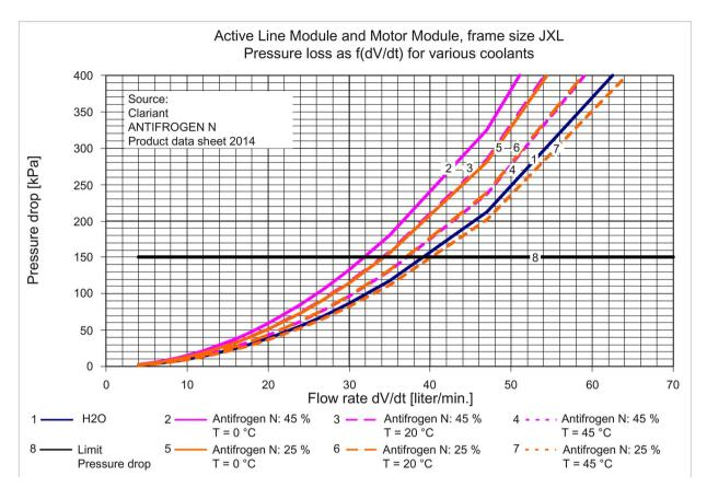
Figure 10-10 Pressure drop as a function of volumetric flow for Active Line Module and Motor Module, frame size JXL
