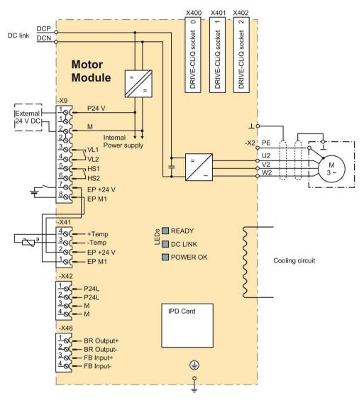
Figure 7-5 Connection example Motor Module
