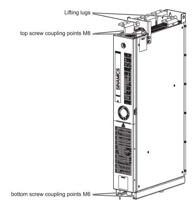
Figure 6-6 Lifting lugs / screw coupling points for mechanical support
