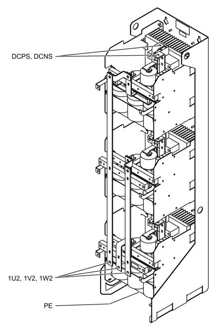
Figure 8-6 Interface overview, voltage peak limiter, type 3
