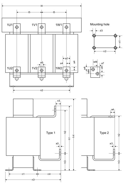
Figure 8-3 Dimension drawing, motor reactor
