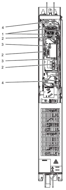
Figure 11-16 Replacing the electronic fan, Active Line Module, and Motor Module, frame size GXL
