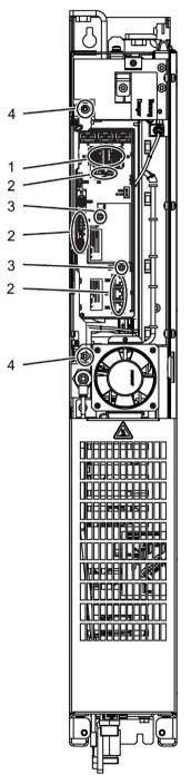
Figure 11-19 Replacing the electronic fan, Basic Line Module, frame size FBL
