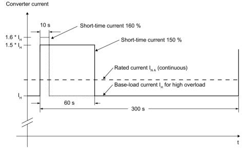
Figure 5-10 High overload
