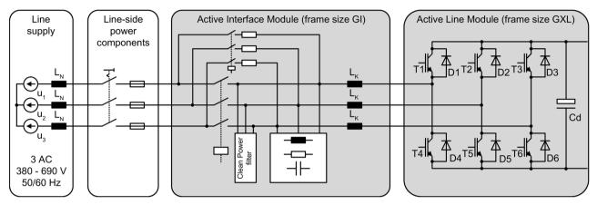
Figure 6-10 Overview of Active Infeeds, frame size GXL
