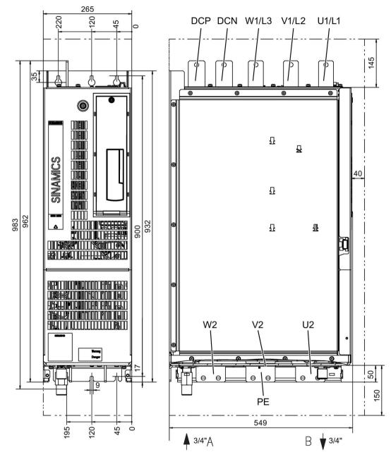
Figure 5-5 Dimension drawing Power Module, frame size GL. Front view, side view
