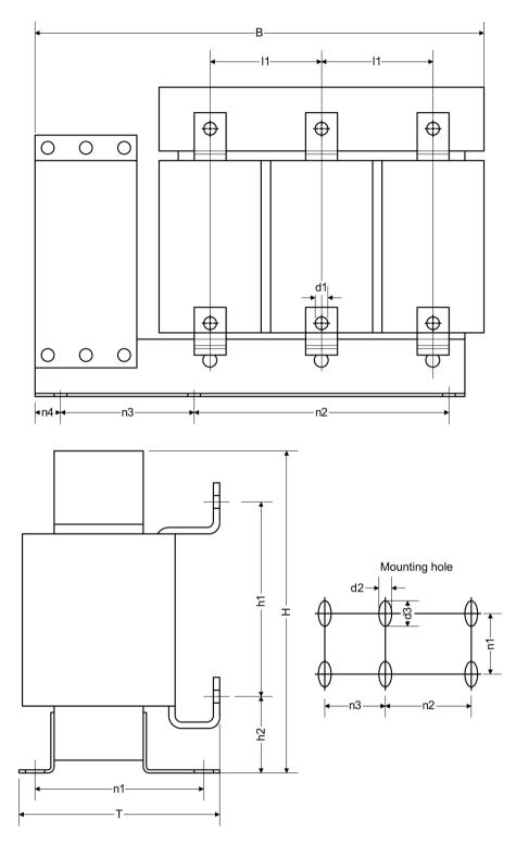
Figure 8-2 Dimension drawing, sine-wave filter
