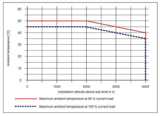
Figure 3-5 Maximum ambient temperature as a function of installation altitude
