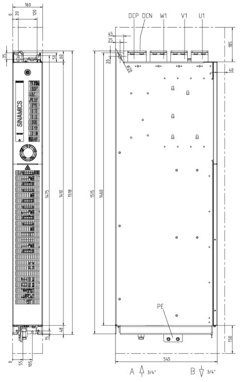
Figure 6-5 Dimension drawing, Basic Line Module, frame size GBL. Front view, side view
