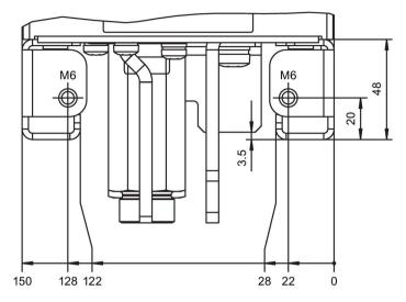
Figure 9-5 Rail profile, Motor Module, frame size FXL (dimensions in mm)
