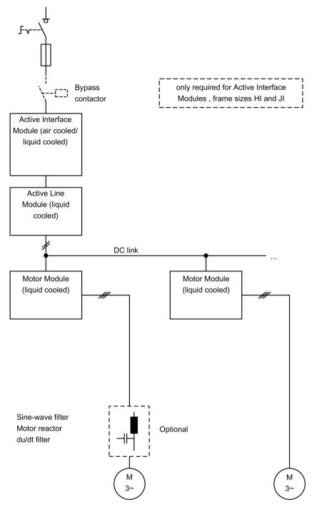
Figure 3-7 Basic structure of a drive system with liquid-cooled SINAMICS S120 and regulated infeed
