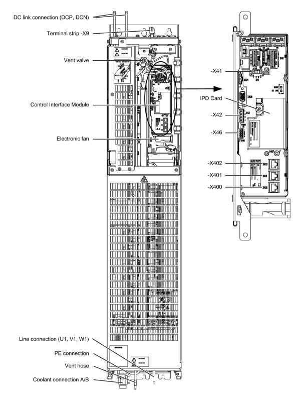
Figure 6-14 Active Line Module, frame size JXL
