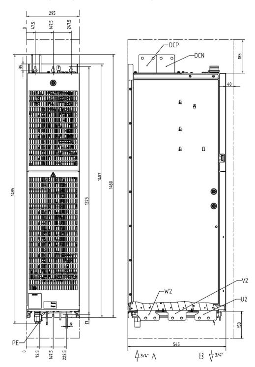
Figure 7-9 Dimension drawing Motor Module, frame size JXL, article numbers 6SL3325-1TE41-0AA3, 6SL3325-1TE41-4AA3, 6SL3325-1TG38-1AA3, 6SL3325-1TG41-0AA3, 6SL3325-1TG41-2AA3, 6SL3325-1TG41-3AA3. Front view, side view
