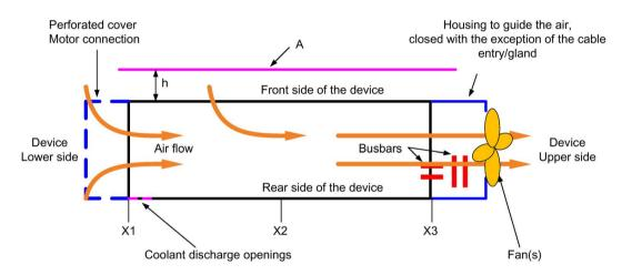
Figure 9-9 Basic layout for horizontal installation position (side view)
