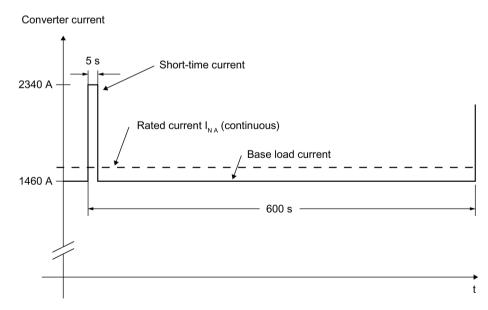
Figure 7-15 High overload for Motor Module 6SL3325-1TG41-6AP3
