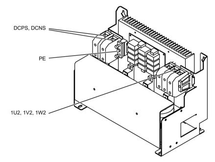
Figure 8-5 Interface overview, voltage peak limiter, type 2
