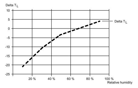
Figure 10-23 Curve to determine the temperature  $\Delta T_{L}$
