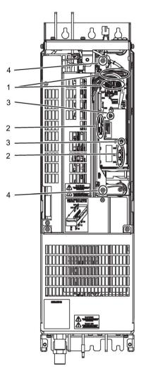
Figure 11-6 Replacing the Control Interface Module, Active Line Module and Motor Module, frame size HXL
