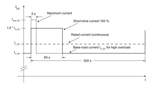
Figure 6-22 High overload
