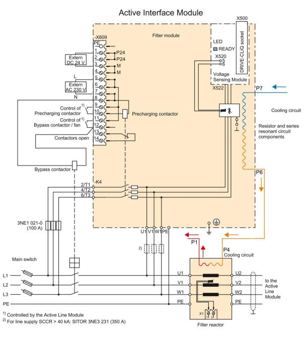
Figure 4-15 Connection example of liquid-cooled Active Interface Module, frame size JIL, valid for article numbers 6SL3305-7TE38-4AA5, 6SL3305-7TG37-4AA5, 6SL3305-7TG41-0AA5 and 6SL3305-7TG41-3AA5
