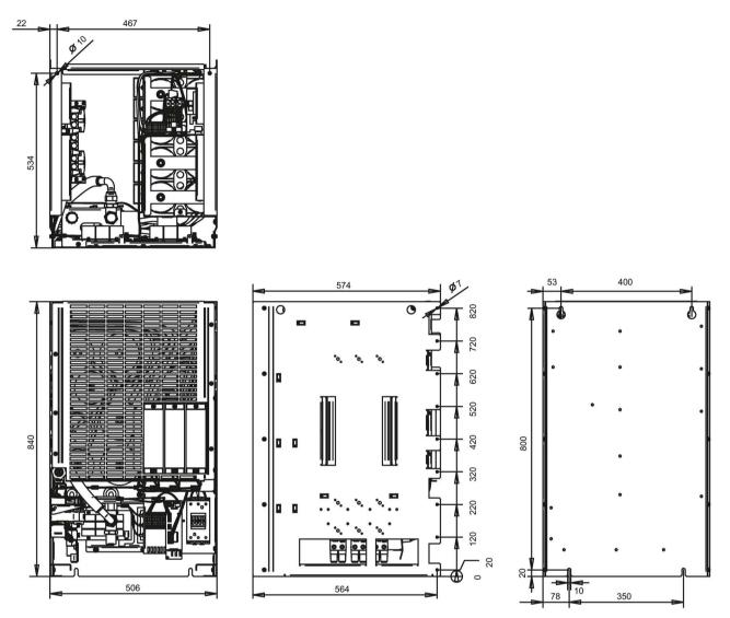
Figure 4-19 Dimension drawing, filter module, frame size JIL
