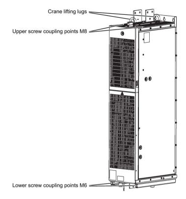
Figure 7-11 Crane lifting lugs / screw coupling points for mechanical support
