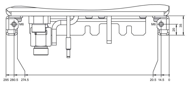
Figure 9-8 Rail profile, Active Line Module and Motor Module, frame size JXL, (dimensions in mm)
