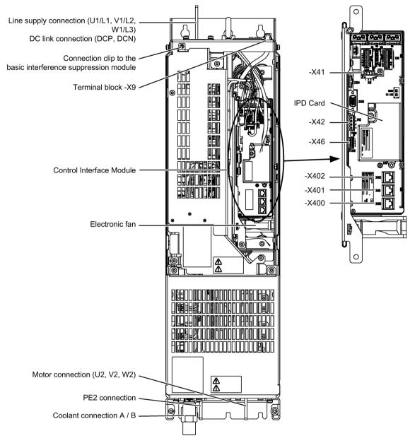
Figure 5-2 Power Module, frame size GL
