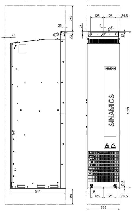
Figure 4-8 Dimension drawing for Active Interface Module, frame size GI Side view, front view
