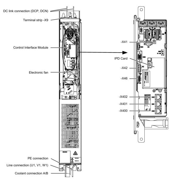
Figure 6-12 Active Line Module, frame size GXL
