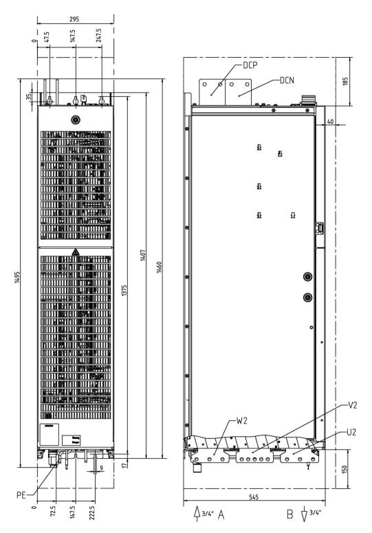
Figure 7-10 Dimension drawing Motor Module, frame size JXL, article numbers 6SL3325-1TE41-4AS3, 6SL3325-1TG41-6AA3. Front view, side view
