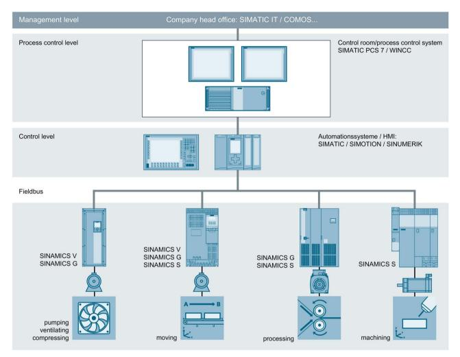
Figure 3-2 SINAMICS in the automation environment
