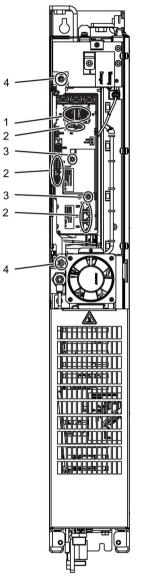
Figure 11-11 Replacing the Control Interface Module, Basic Line Module, frame size FBL
