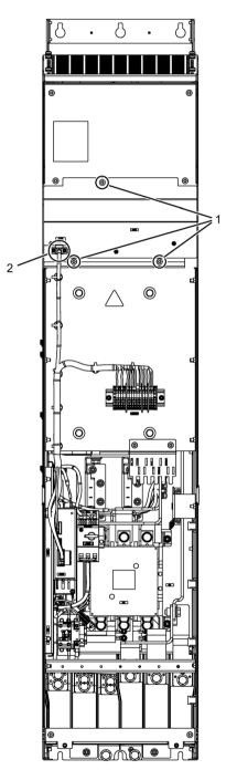
Figure 11-22 Replacing the fan, Active Interface Module, frame size GI
