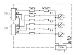
Figure 4-7 Internal circuit of the VSM10 Voltage Sensing Module
