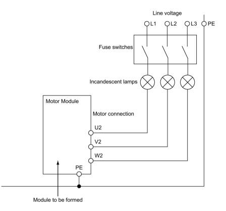
Figure 11-26 Forming circuit for Motor Modules
