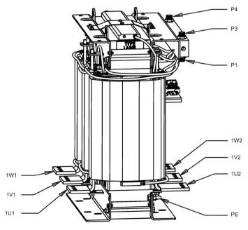
Figure 4-14 Interface overview filter reactor, frame size JIL, valid for article numbers 6SL3005-0DE41-4AA0 and 6SL3005-0DG41-6AA0
