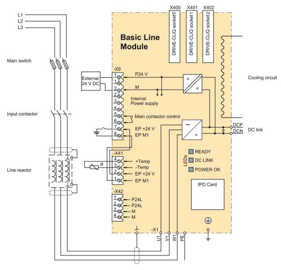
Figure 6-3 Connection example for Basic Line Modules
