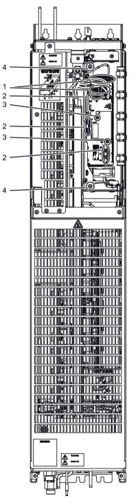
Figure 11-8 Replacing the Control Interface Module, 6SL3325-1TG41-6AP3 Motor Module
