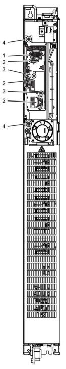
Figure 11-12 Replacing the Control Interface Module, Basic Line Module, frame size GBL
