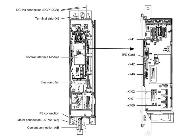
Figure 7-1 Motor Module, frame size FXL
