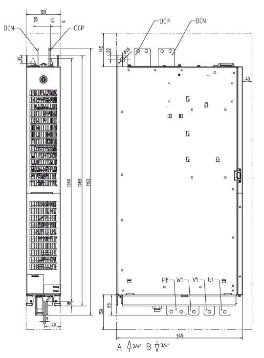
Figure 6-16 Dimension drawing Active Line Module, frame size GXL Front view, side view
