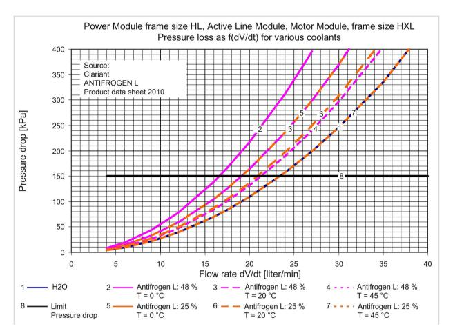
Figure 10-17 Pressure drop as a function of flow rate for Power Module frame size HL, Active Line Module and Motor Module frame size HXL
