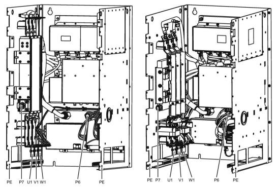
Interface overview filter module, size JIL, valid Interface overview filter module, size JIL, valid for function release  $FS \neq 03$  for function release FS = 03
