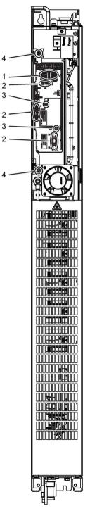
Figure 11-20 Replacing the electronic fan, Basic Line Module, frame size GBL
