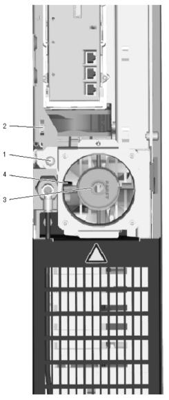
Figure 10-27 Removing the electronics fan to actuate the vent valve
