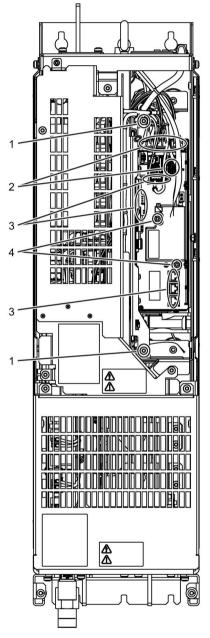
Figure 11-14 Replacing the electronic fan, Power Module, frame size GL
