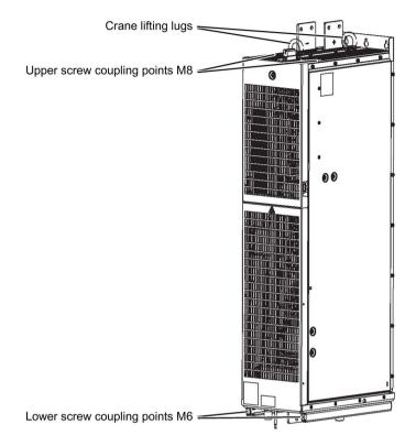
Figure 6-20 Crane lifting lugs / screw coupling points for mechanical support
