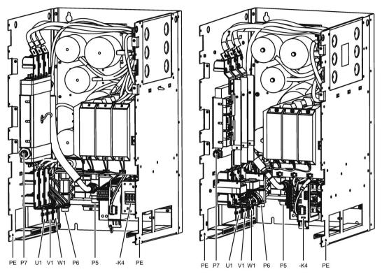
Interface overview filter module, size JIL, valid Interface overview filter module, size JIL, valid for function release FS ≠ 03 for function release FS = 03
