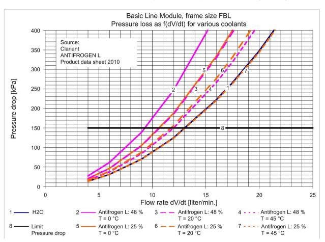
The following diagrams show the pressure drop as a function of the volumetric flow rates for the different SINAMICS S120 liquid-cooled components when using Antifrogen L.
