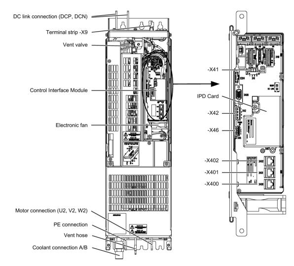
Figure 7-3 Motor Module, frame size HXL
