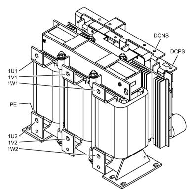
Figure 8-15 Interface overview for dv/dt filter compact plus Voltage Peak Limiter, Type 3
