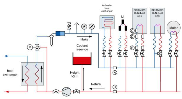
Figure 10-3 Arrangement of pressure compensator, component pressure drops
