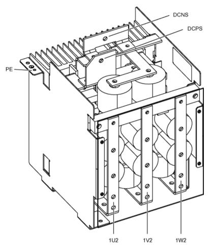
Figure 8-17 Interface overview for dv/dt filter compact plus Voltage Peak Limiter, Type 4 Voltage Peak Limiter
