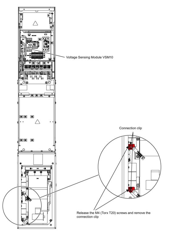
Figure 4-12 Removing the connection clip of the basic interference suppression module to ground for frame size HI
