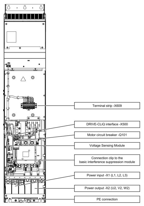
Figure 4-3 Interface overview in the Active Interface Module, frame size GI
