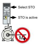
The converter with active STO function prevents energy supply to the motor. The motor can no longer generate torque on the motor shaft.
