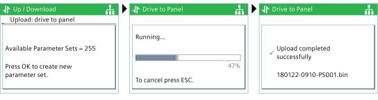
The number of available parameter sets are displayed The drive parameter settings are uploaded
