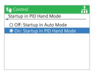
Select On: Startup in PID Hand Mode
