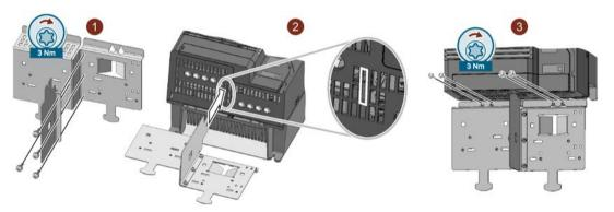
Use the shield plate provided for strain relief of the line and motor cable – as well as the shield support for the motor cable.
