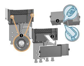
FSF, FSG: Remove the lower cover
