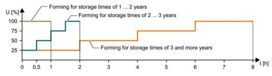
Figure 5-2 Forming the DC-link capacitors
