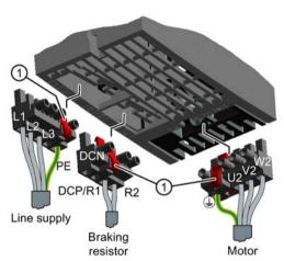
The Power Modules are equipped with withdrawable plug connectors that cannot be inadvertently interchanged.
