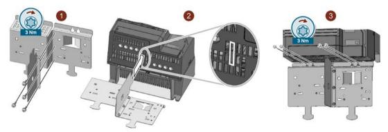
You have correctly mounted the EMC connecting bracket and the shield plate.
