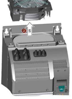
2. Install the new fan module in inverse sequence.
