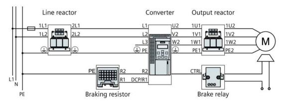
Figure 4-7 Connecting the PM240-2 Power Module, 200 V 1 AC, FSA ... FSC
