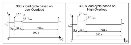
Figure 6-1 "Low Overload" and "High Overload" load cycles
