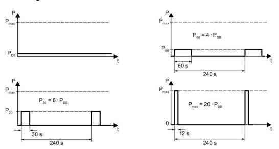
Figure 8-5 Pulse power, rated power and examples of the switch-on duration of the braking resistor
