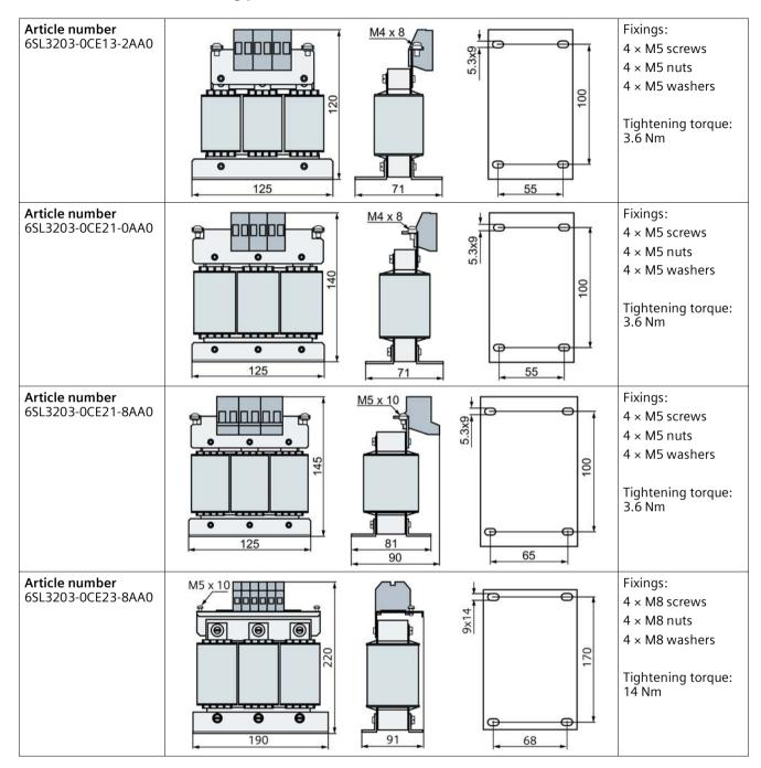
Assignment of line reactor to converter:
