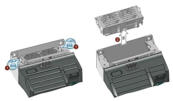
2. Install the new fan module in inverse sequence. By inserting the fan module, you establish the electrical connection between the converter and fan module.
