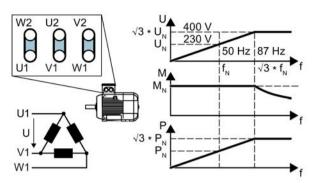
In a delta connection, the motor is operated with a voltage and frequency above its rated values. As a consequence, the motor power is increased by a factor  $\sqrt{3} \approx 1.73$ .
