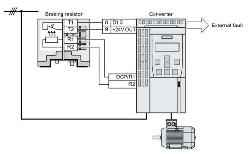
Figure 8-3 Connecting a braking resistor with temperature monitoring via digital input DI 3
