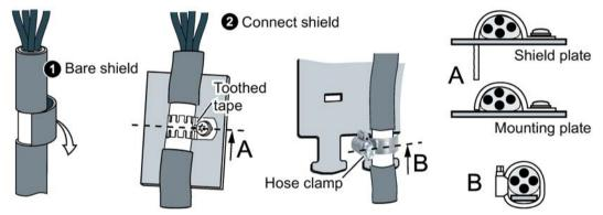
Figure 3-4 Examples for EMC-compliant shield support
