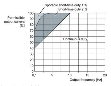
Figure 6-2 Permissible operating range of the converter
