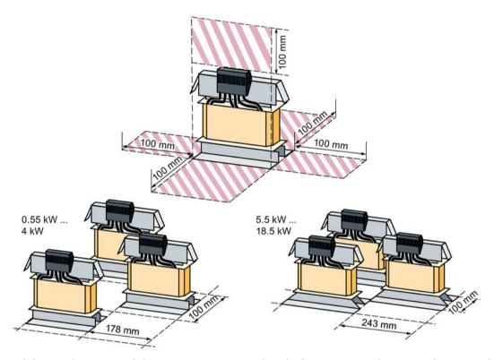
Minimum clearances of the output reactor to other devices, space-saving mounting examples
