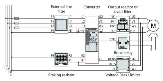
Figure 4-6 Connecting the PM240-2 Power Module, 200 V / 400 V / 690 V 3 AC, FSD ... FSG
