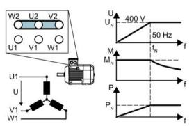
In a star connection, the motor can provide its rated torque Mn in the range 0 ... rated frequency f<sub>N</sub>.
