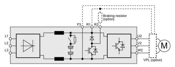
Figure 4-4 Block diagram for the converter, FSD ... FSG
