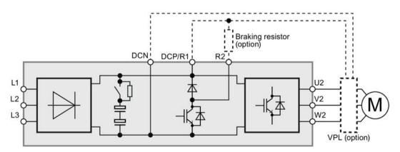
Figure 4-3 Block diagram of the converter, FSA ... FSC
