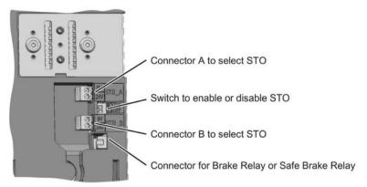
Figure 4-9 Terminals and switches for the "STO via power module terminals" function
