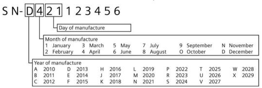
Figure 5-1 Data of manufacture in the serial number (example, April 21, 2013)
