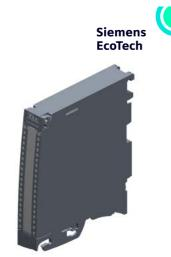
SIMATIC S7-1500 Analog input/output module AI 4x U/I/R/RTD/TC ST; 4 channels in groups of 4; Hardware interrupts; Diagnostics AQ 2x U/I ST; 2 channels in groups of 2; Substitute value; Diagnostics Common mode voltage approx. 10 V 16 bit; Accuracy 0.3%; Delivery including push-in front connector, infeed element, shield bracket and shield terminal
