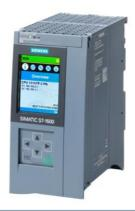
SIMATIC S7-1500T, CPU 1515TF-2 PN, central processing unit with 1.5 MB work memory for program and 4.5 MB for data, 1st interface: PROFINET IRT with 2-port switch, 2nd interface: PROFINET RT, 6 ns bit performance, SIMATIC Memory Card required - - - approvals and certificates according to entry 109816881 at support.industry.siemens.com to be considered! - -
