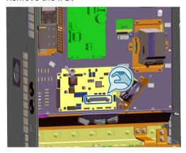
5. Remove the 6 screws on the FPI board (torx 20).
