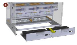
5. Install the new fan unit(s) in the reverse sequence (tightening torque for the fixing screws: 3 Nm/26.5 lbf.in).
