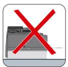
Figure 3-1 Only mount in the vertical position with the line connection at the bottom
