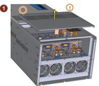
3. Disconnect the two cable lugs of fan power supply (2).
