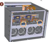
4. Release the retaining screws (four screws on FSH, and eight screws on FSJ) ③ and draw out the fan unit(s) ④.
