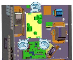
3. Remove the connectors on the power supply board.
