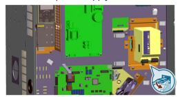
The power supply is removed.
