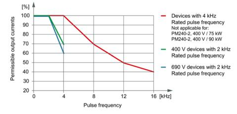
Figure 5-29 Reduction of the output current as a function of the pulse frequency
