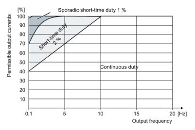
Figure 5-48 Reduction of the output current as a function of the output frequency
