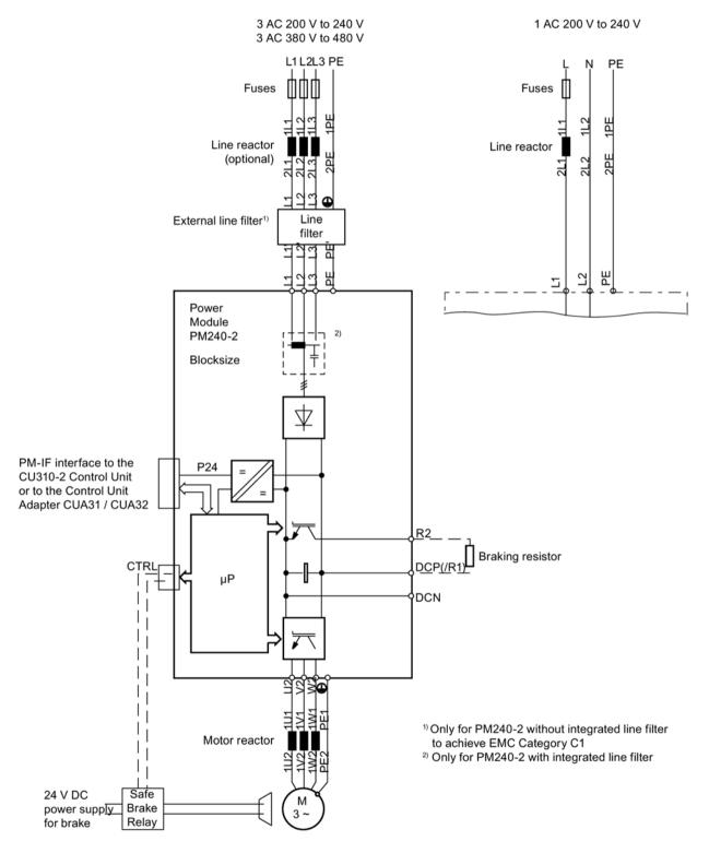
Figure 5-8 Connection example, Power Modules PM240-2, FSA-FSC
