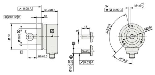
Figure 9-22 Dimension drawing of clamping flange, all data in mm
