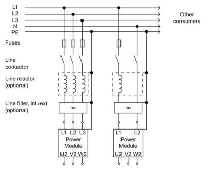
Figure 4-19 Direct operation on the line supply
