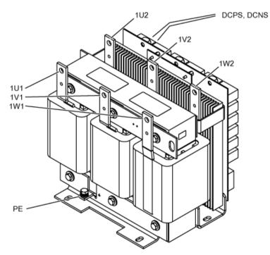
Figure 7-16 Interface overview, dV/dt filter compact plus Voltage Peak Limiter, type 2
