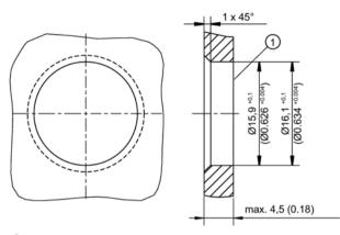
① Through-hole with chamfer
