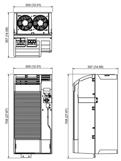
Figure 5-15 Dimension drawing of PM240-2 Power Modules, frame size FSF, all data in mm (inches)
