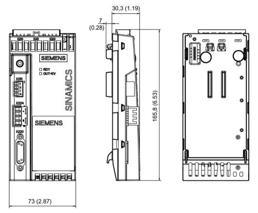
Figure 8-21 Dimension drawing of Control Unit Adapter CUA32, all data in mm and (inches)
