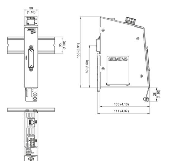
Figure 9-2 Dimension drawing of the Sensor Module Cabinet SMC10, all dimensions in mm and (inches)
