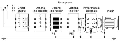
Figure 4-1 Example of a Blocksize line connection (FSA to FSC)
