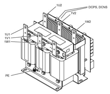
Figure 7-15 Interface overview, dV/dt filter compact plus Voltage Peak Limiter, type 1
