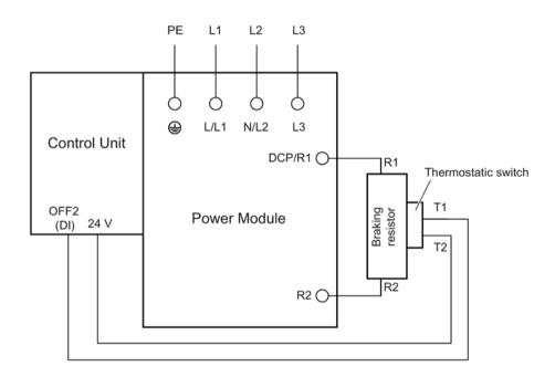
Figure 6-1 Connecting the thermostatic switch on the braking resistor to a Control Unit
