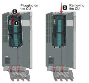
Figure 8-22 Mounting (left) and removal (right) of the Control Unit
