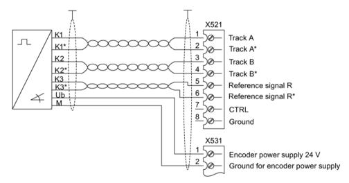
Figure 9-10 Connection example 1: HTL encoder, bipolar, with reference signal
