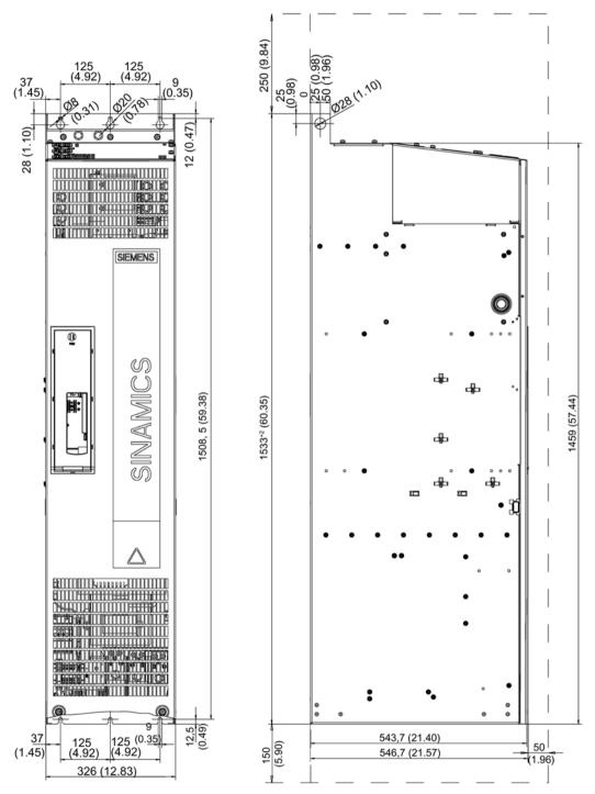
Figure 5-45 Dimension drawing Power Module, frame size GX
