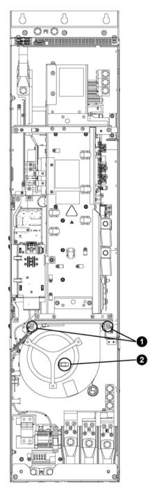
Figure 12-9 Replacing the fan, Power Module, frame size FX
