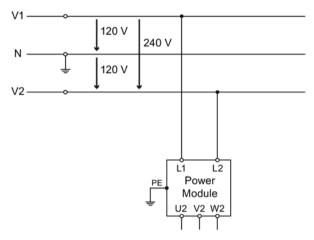
Figure 4-20 Direct operation on single phase grounded midpoint line system configurations
