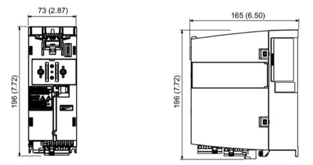
Figure 5-10 Dimension drawing of PM240-2 Power Modules, frame size FSA, all data in mm (inches)
