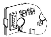
Figure 8-3 CU310-2 PN interface to the Power Module (PM-IF)
