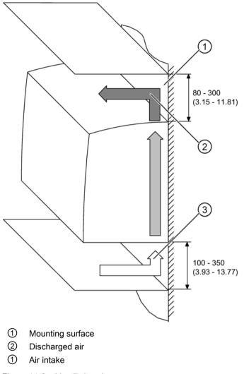
Figure 11-6 Ventilation clearances
