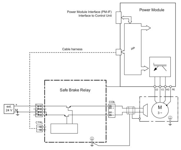
Figure 9-30 Safe Brake Relay connection example
