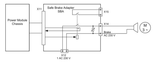
Figure 9-33 Connection example for a Safe Brake Adapter
