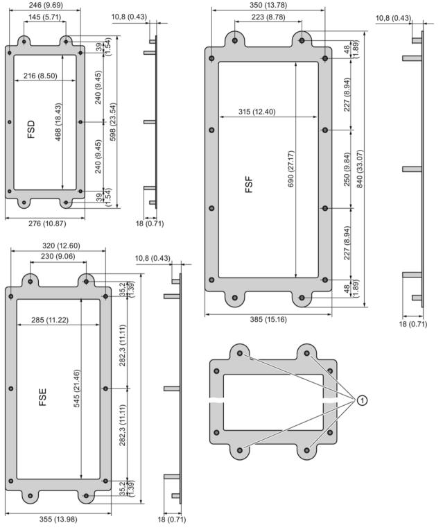
① Bolts for mounting onto the electrical cabinet panel
