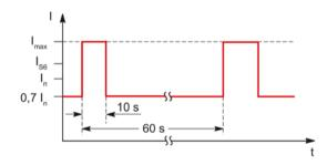
Figure 5-38 S6 peak current load cycle with pre-load condition
