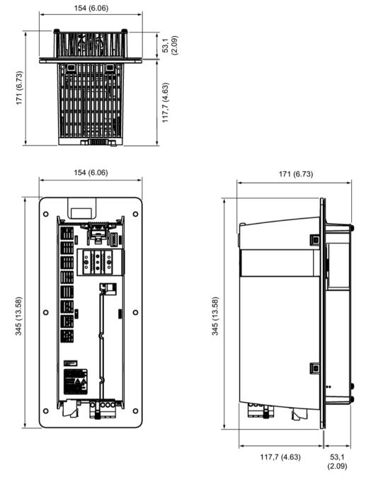
Figure 5-19 Dimension drawing of PM240-2 Push Through Power Modules, frame size FSB, all data in mm (inches)
