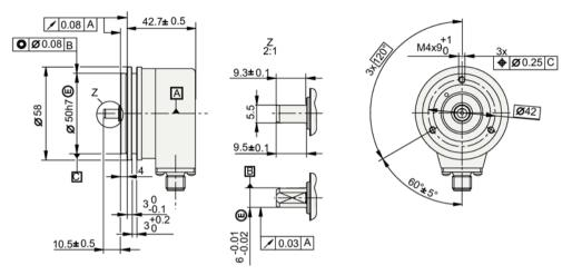
Figure 9-21 Dimension drawing of synchro flange, all data in mm
