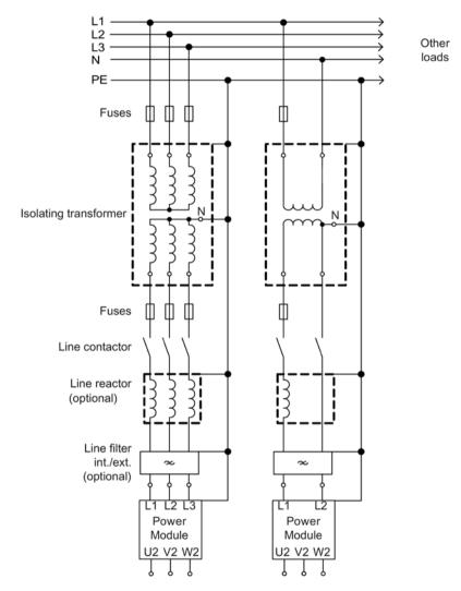
Figure 4-22 Connecting to the line supply using an isolating transformer
