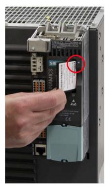
Figure 8-5 CU310-2 PN Inserting the memory card
