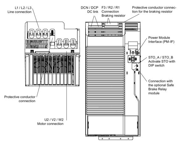
Figure 5-6 PM240-2, frame size FSF (view from below and front)
