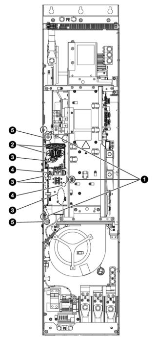
Figure 12-7 Replacing the Control Interface Module, Power Module, frame size FX
