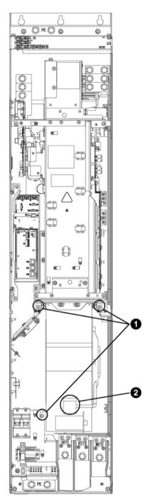
Figure 12-10 Replacing the fan, Power Module, frame size GX
