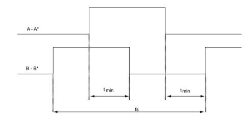
Figure 9-18 Signal characteristic of track A and track B between two edges: Time between two edges with pulse encoders
