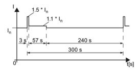
Figure 5-33 300 s load cycle based on Low Overload
