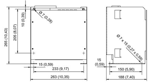
Figure 7-13 Dimension drawing of the Voltage Peak Limiter, type 1
