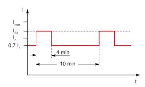
Figure 5-37 S6 duty cycle with pre-load condition
