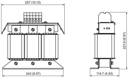
Figure 7-3 Dimension drawing, motor reactor 6SL3202-0AE23-8CA0, all data in mm and (inch)
