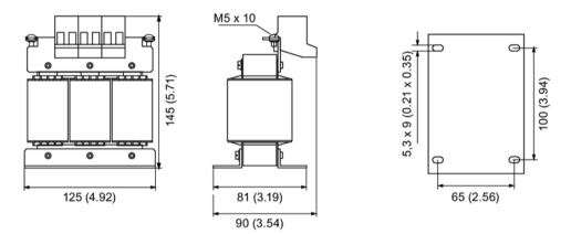
Figure 4-11 Dimensional drawing of line reactors, PM240-2, frame size FSB, 4.0 ... 7.5 kW, all dimensions in mm and (inch)
