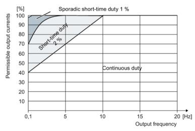
Figure 5-32 Reduction of the output current as a function of the output frequency
