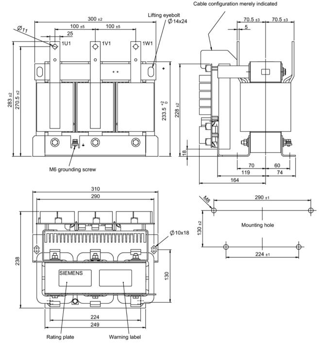
dV/dt filter compact plus Voltage Peak Limiter, type 1
