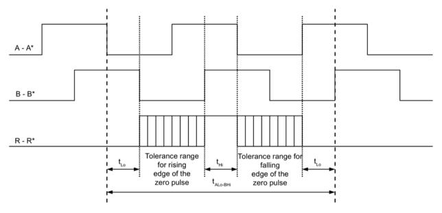
Figure 9-19 Position of the zero pulse to the track signals
