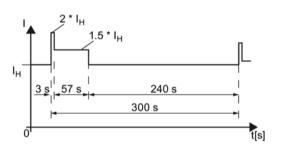
Figure 5-34 300 s load cycle based on High Overload
