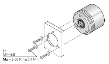
Figure 9-24 Installation: Synchro flange
