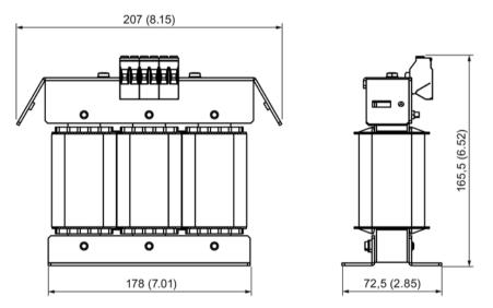
Figure 7-1 Dimension drawing, motor reactors 6SL3202-0AE16-1CA0 and 6SL3202-0AE18-8CA0, all data in mm and (inch)
