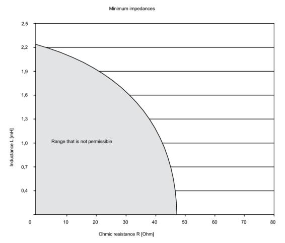
Figure 9-4 Rotor impedances that can be connected with excitation frequency f = 5000 Hz
