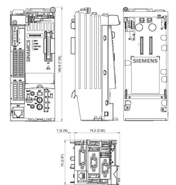
Figure 8-15 Dimension drawing, Control Unit CU310-2 DP, all data in mm (inches)
