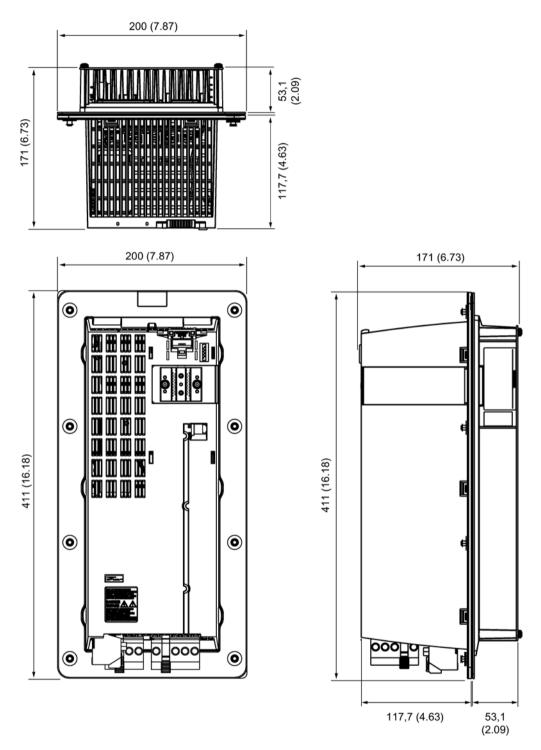
Figure 5-20 Dimension drawing of PM240-2 Push Through Power Modules, frame size FSC, all data in mm (inches)
