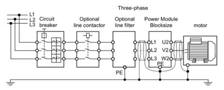
Figure 4-2 Example of a blocksize line connection (FSD to FSG)
