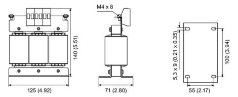
Figure 4-10 Dimensional drawing of line reactors, PM240-2 frame size FSA, 1.5 ... 4.0 kW, all dimensions in mm and (inch)
