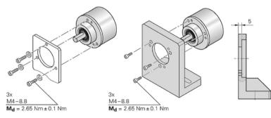
Figure 9-26 Installation: Clamp flange with axial screws
