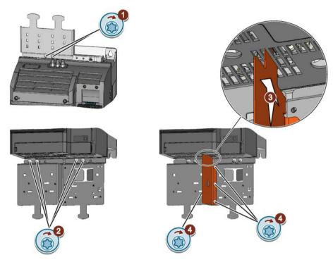
Figure 5-23 Mounting a shield connection plate onto a PM240-2 Power Module, FSD and FSE
