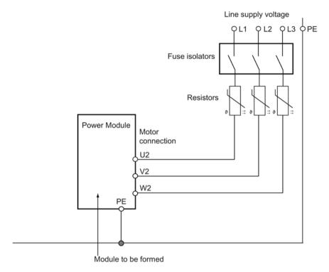
Figure 12-12 Forming circuit for 3-phase AC Power Modules with resistors
