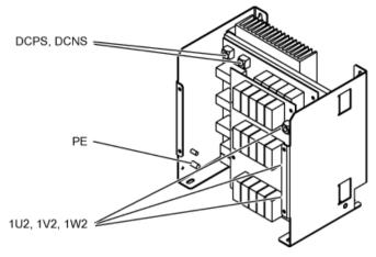
Figure 7-9 Interface overview, Voltage Peak Limiter, type 1
