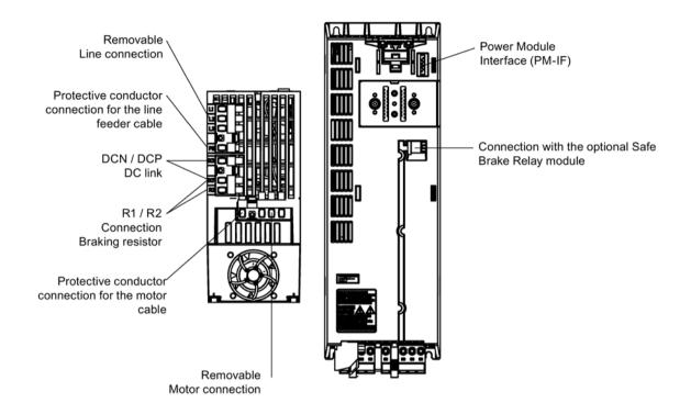
Figure 5-2 PM240-2, frame size FSB (view from below and front)
