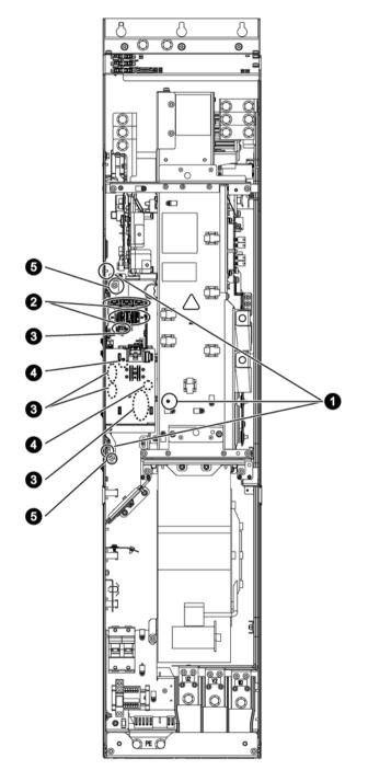
Figure 12-8 Replacing the Control Interface Module, Power Module, frame size GX
