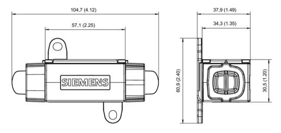
Figure 10-11 Dimension drawing of the DRIVE-CLiQ coupling, all dimensions in mm and (inches)
