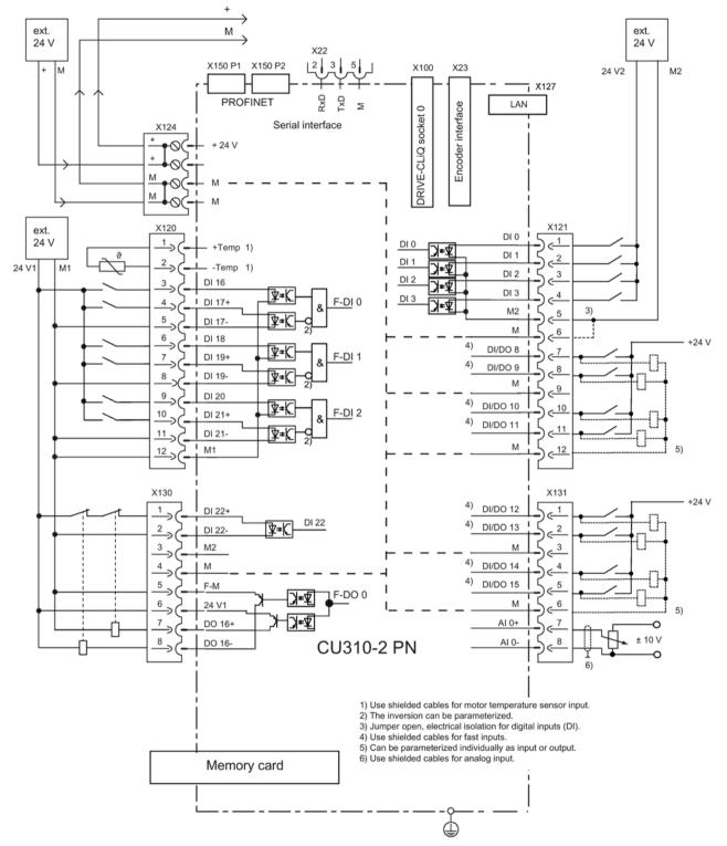
Figure 8-7 Connection example, CU310-2 PN with safety function
