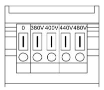
Figure 5-46 Setting terminals for the fan transformers
