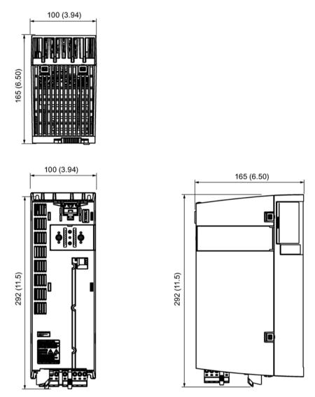
Figure 5-11 Dimension drawing of PM240-2 Power Modules, frame size FSB, all data in mm (inches)
