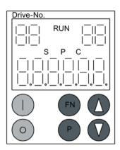
Figure 8-24 Overview of displays and keys
