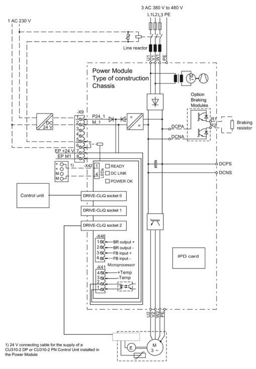
Figure 5-43 Connection example: Power Module chassis
