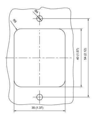
Figure 10-5 Cutout in the control cabinet, all dimensions in mm and (inches)
