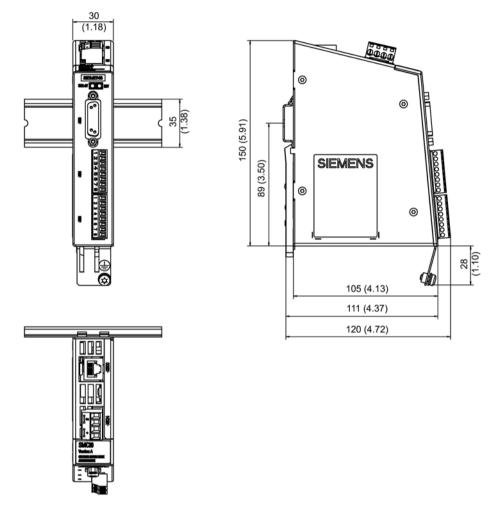
Figure 9-13 Dimension drawing of the Sensor Module Cabinet SMC30, all data in mm and (inches)
