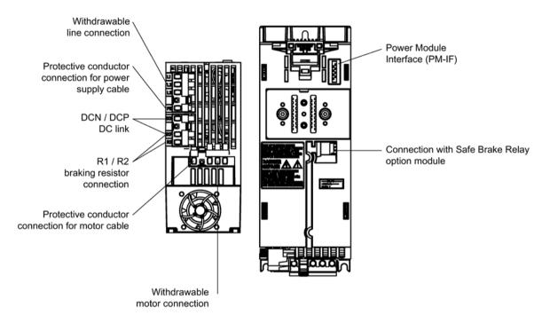
Figure 5-1 PM240-2, frame size FSA (view from below and front)
