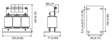
Figure 4-9 Dimensional drawing of line reactors, PM240-2 frame size FSA, 0.55 ... 1.1 kW, all dimensions in mm and (inch)
