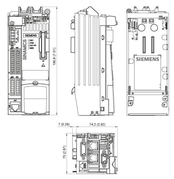
Figure 8-8 Dimension drawing, Control Unit CU310-2 PN, all data in mm (inches)
