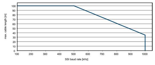
Figure 8-4 Maximum cable lengths depending on the SSI baud rate for SSI encoders
