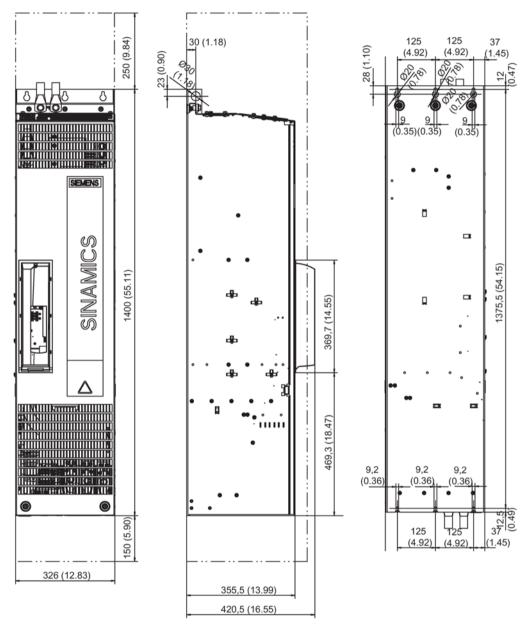
Figure 5-44 Dimension drawing Power Module, frame size FX
