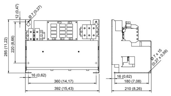
Figure 7-14 Dimension drawing of the Voltage Peak Limiter, type 2
