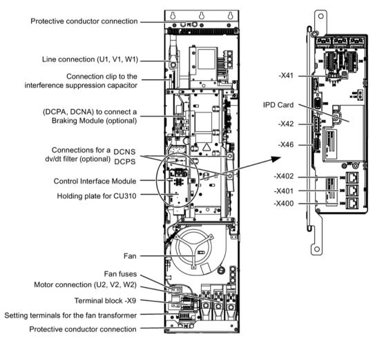
Figure 5-41 Power Module, frame size FX
