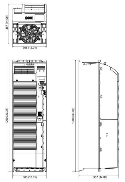
Figure 5-16 Dimension drawing of PM240-2 Power Modules, frame size FSG, all data in mm (inches)
