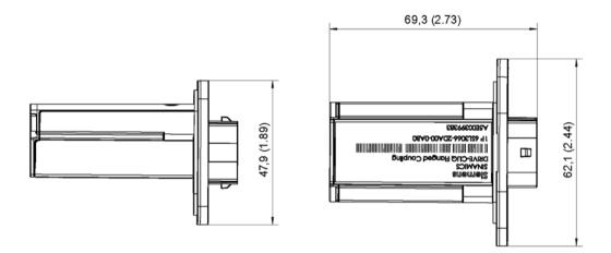
Figure 10-3 Dimension drawing of the DRIVE-CLiQ cabinet gland, all dimensions in mm and (inches)
