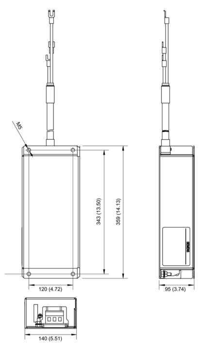
Figure 4-6 Dimension drawing of the line filter, Power Module PM240-2 frame size FSC, all data in mm (inches)
