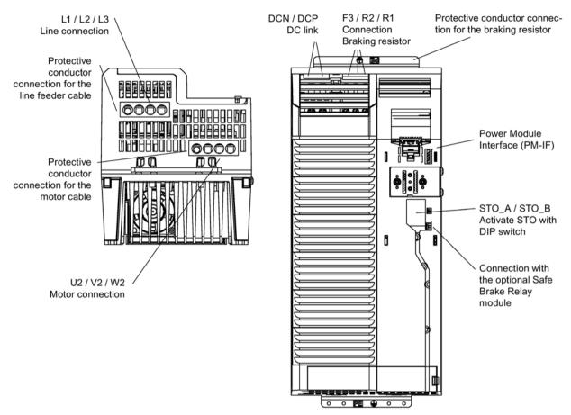
Figure 5-4 PM240-2, frame size FSD (view from below and front)
