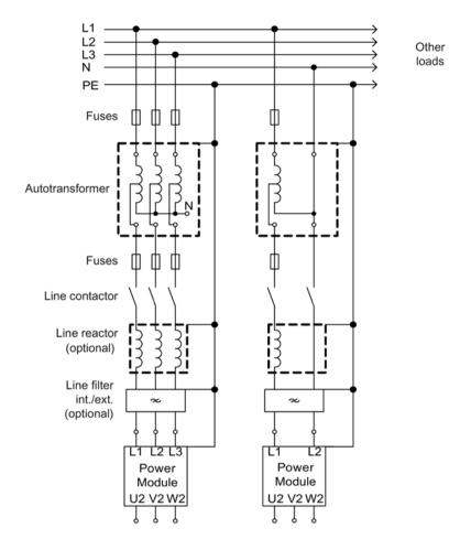
Figure 4-21 Connecting to the line supply using an autotransformer
