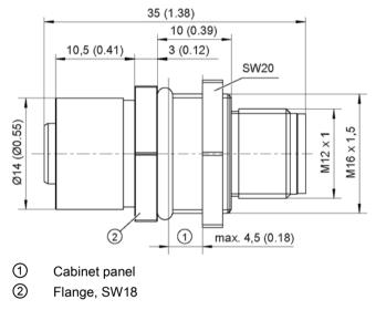
Figure 10-4 Dimension drawing of the DRIVE-CLiQ cabinet bushing M12, all dimensions in mm and (inches)
