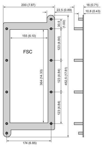
Figure 10-14 Dimension drawing of mounting frame, frame size FSC, all data in mm and (inches)
