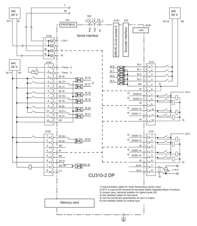
Figure 8-13 Connection example, CU310-2 DP without safety function
