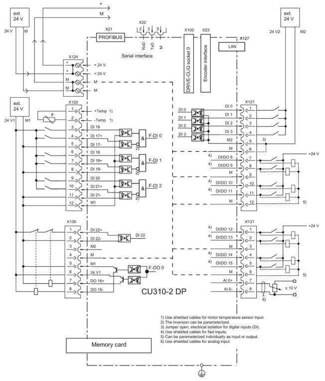
Figure 8-14 Connection example, CU310-2 DP with safety function
