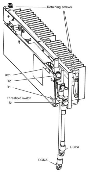
Figure 6-5 Braking Module for Power Module, frame size GX
