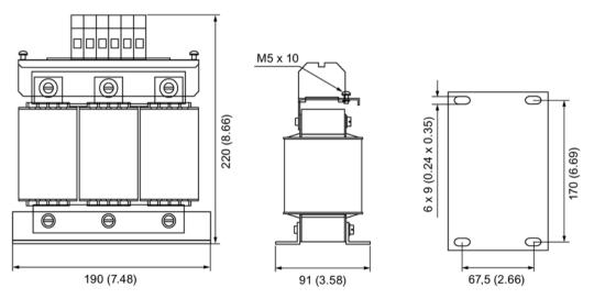
Figure 4-12 Dimensional drawing of line reactors, PM240-2, frame size FSC, 11 ... 15 kW, all dimensions in mm and (inch)
