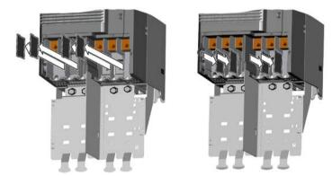
Figure 5-27 PM240-2, FSG, insulating plates
