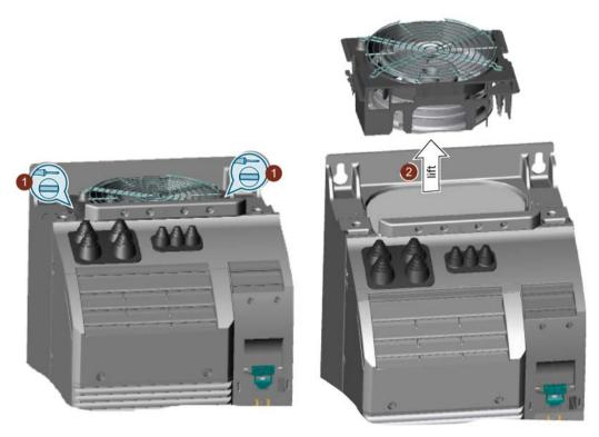
Figure 12-3 Fan replacement PM240-2, frame size FSG
