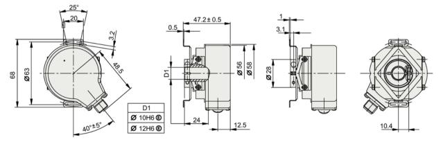
Figure 9-23 Dimension drawing of hollow shaft, all data in mm
