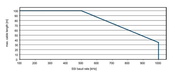
Figure 9-8 Maximum cable lengths depending on the SSI baud rate for SSI encoders
