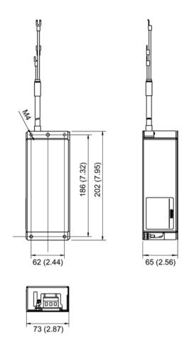
Figure 4-4 Dimension drawing of the line filter, Power Module PM240-2 frame size FSA, all data in mm (inches)
