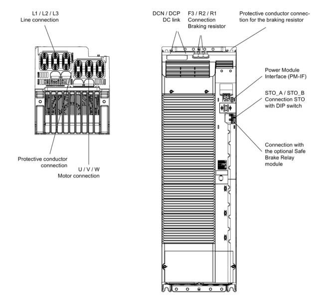
Figure 5-7 PM240-2, frame size FSG (view from below and front)
