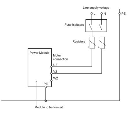
Figure 12-13 Forming circuit for 1-phase AC Power Modules with resistors
