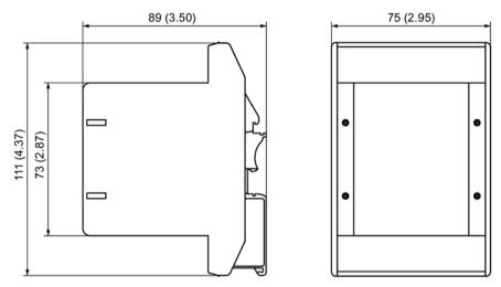
Figure 9-34 Dimension drawing of Safe Brake Adapter, all data in mm and (inches)
