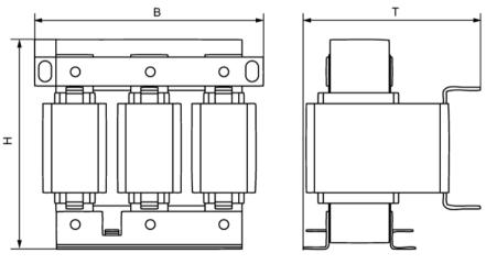
Figure 7-4 Dimension drawing of 6SE4000-3TC..-..D0 motor reactor, dimensions, see the following table
