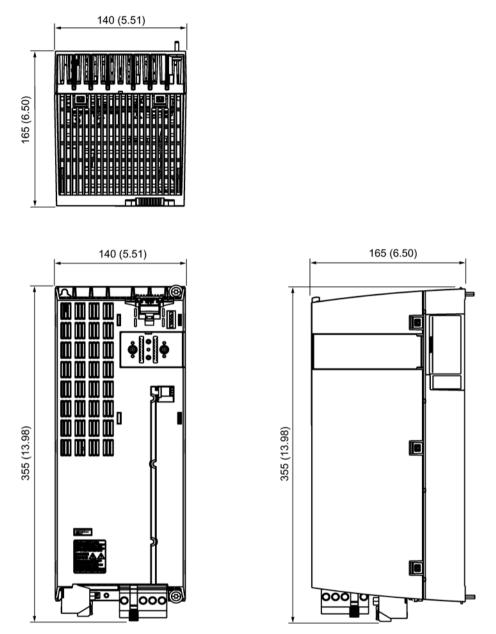
Figure 5-12 Dimension drawing of PM240-2 Power Modules, frame size FSC, all data in mm (inches)
