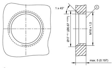
① Threaded hole with chamfer
