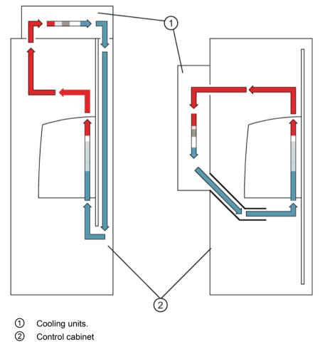
Figure 11-7 Examples of cabinet ventilation
