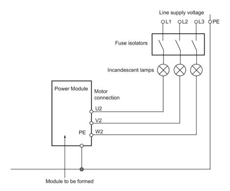
Figure 12-11 Forming circuit for 3-phase AC Power Modules with incandescent lamps
