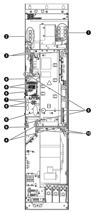
Figure 12-6 Replacing the Powerblock, Power Module, frame size GX
