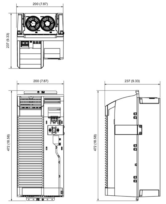
Figure 5-13 Dimension drawing of PM240-2 Power Modules, frame size FSD, all data in mm (inches)
