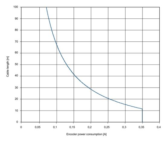
Figure 9-17 Max. cable length as a function of the encoder current drawn
