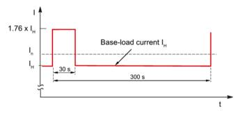
Figure 5-40 Duty cycle with 30 s overload with a duty cycle duration of 300 s
