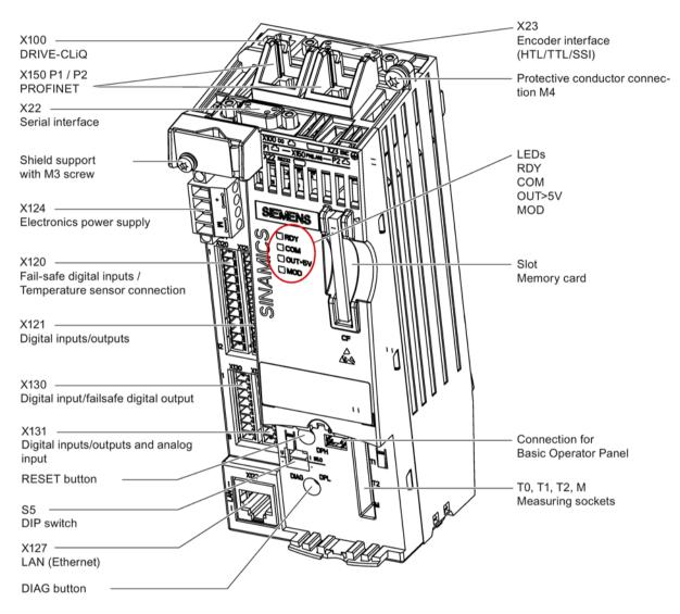
Figure 8-2 CU310-2 PN overview of interfaces
