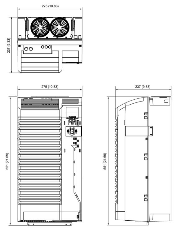
Figure 5-14 Dimension drawing of PM240-2 Power Modules, frame size FSE, all data in mm (inches)
