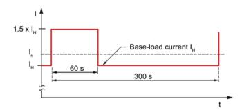
Figure 5-39 Duty cycle with 60 s overload with a duty cycle duration of 300 s
