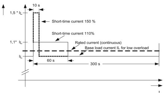
Figure 5-49 Characteristic: Low overload
