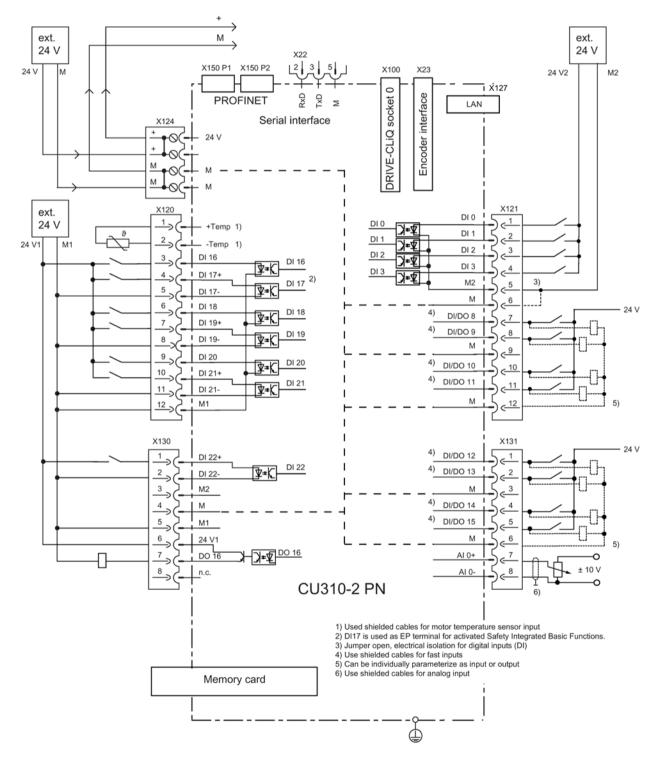
Figure 8-6 Connection example, CU310-2 PN without safety function
