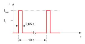
Figure 5-36 Duty cycle without initial load (for servo drives)
