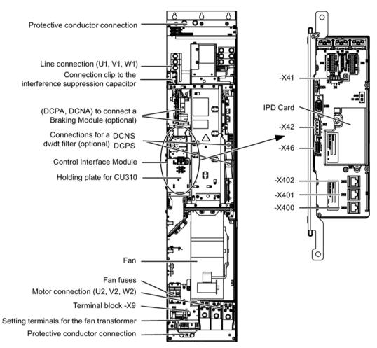
Figure 5-42 Power Module, frame size GX
