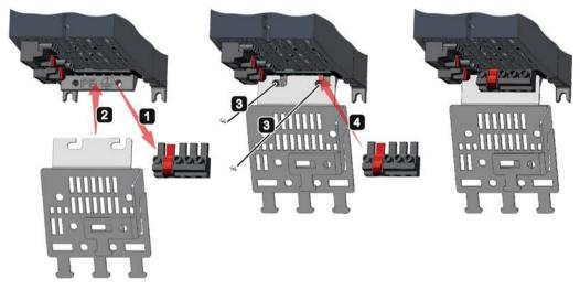
Figure 5-22 Mounting a shield connection plate onto a PM240-2 Power Module, FSA to FSC
