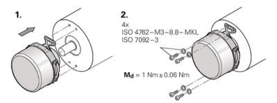
Figure 9-28 Installation: Hollow shaft
