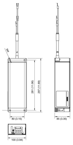
Figure 4-5 Dimension drawing of the line filter, Power Module PM240-2 frame size FSB, all data in mm (inches)
