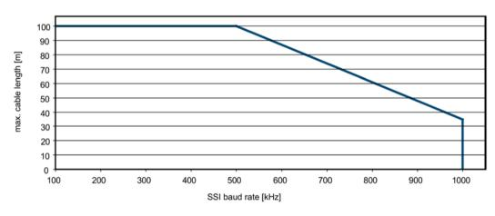
Figure 8-11 Maximum cable lengths depending on the SSI baud rate for SSI encoders
