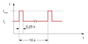
Figure 5-35 Duty cycle with initial load (for servo drives)
