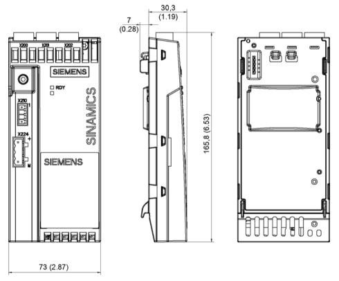
Figure 8-18 Dimension drawing of Control Unit Adapter CUA31, all data in mm and (inches)
