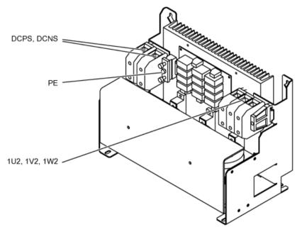
Figure 7-10 Interface overview, Voltage Peak Limiter, type 2
