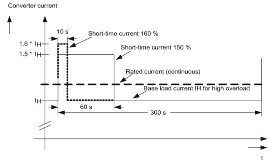
Figure 5-50 Characteristic: High overload
