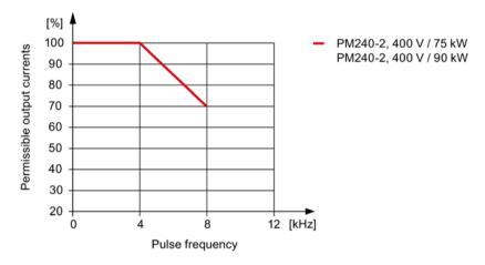
Figure 5-30 Reduction of the output current as a function of the pulse frequency (for PM240-2; 400 V, 75 and 90 kW)
