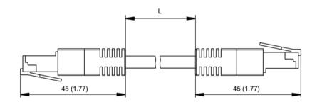
Figure 11-2 DRIVE-CLiQ signal cables without 24 V DC cores (IP20)
