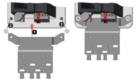
Figure 5-26 Mounting a shield connection plate onto a push through PM240-2 Power Module, FSA to FSC
