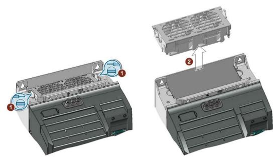
Figure 12-2 Fan replacement PM240-2, frame sizes FSD ... FSF
