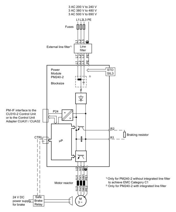
Figure 5-9 Connection example, Power Modules PM240-2, FSD-FSG
