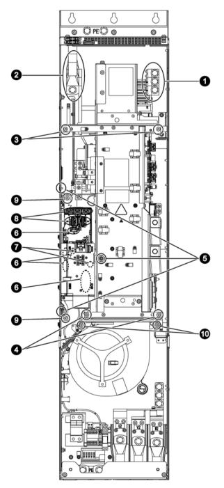
Figure 12-5 Replacing the Powerblock, Power Module, frame size FX
