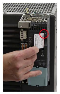
Figure 8-12 CU310-2 DP Inserting the memory card
