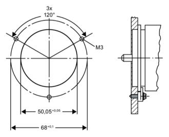
Figure 9-25 Installation with clamp straps
