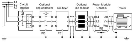
Figure 4-3 Example of a chassis line connection
