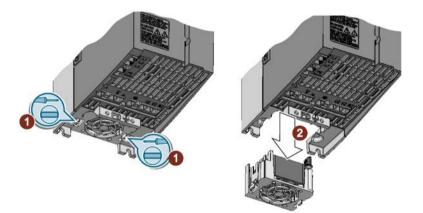
Figure 12-1 Fan replacement PM240-2, frame sizes FSA ... FSC
