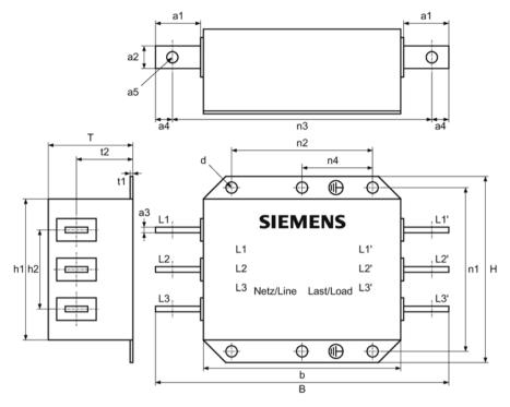
Figure 4-7 Dimension drawing, line filter
