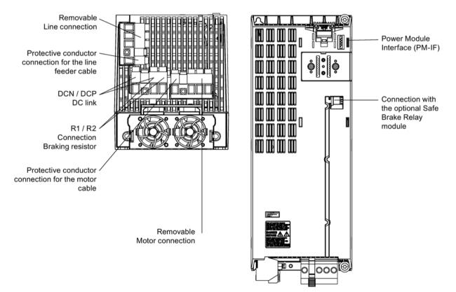
Figure 5-3 PM240-2, frame size FSC (view from below and front)
