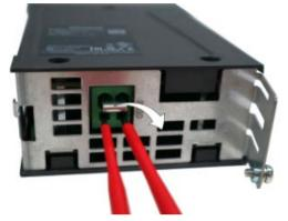
Terminal X530 with connector jumper
