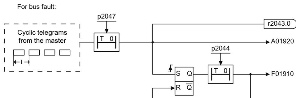
Figure 5-5 Monitoring telegram failure with a bus fault
