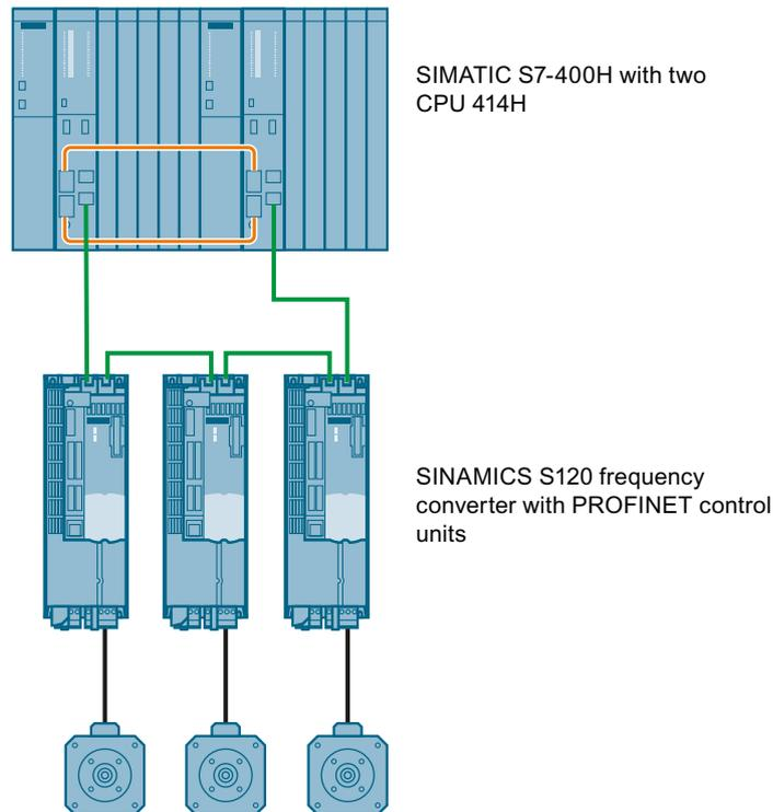
Figure 6-18 System redundancy with converters
