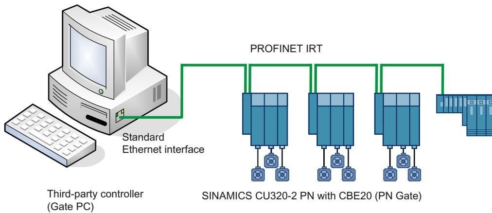
Figure 6-4 Schematic representation of SINAMICS PROFINET Gate (in short: PN Gate)
