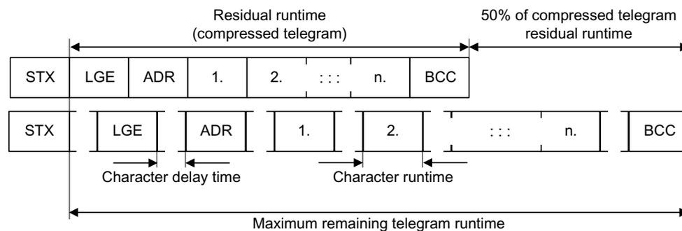
Figure 10-8 Telegram runtime as the sum of the residual runtime and character delay times
