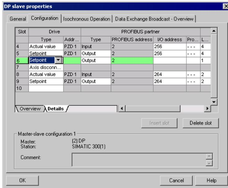
Figure 5-13 Insert new slot
