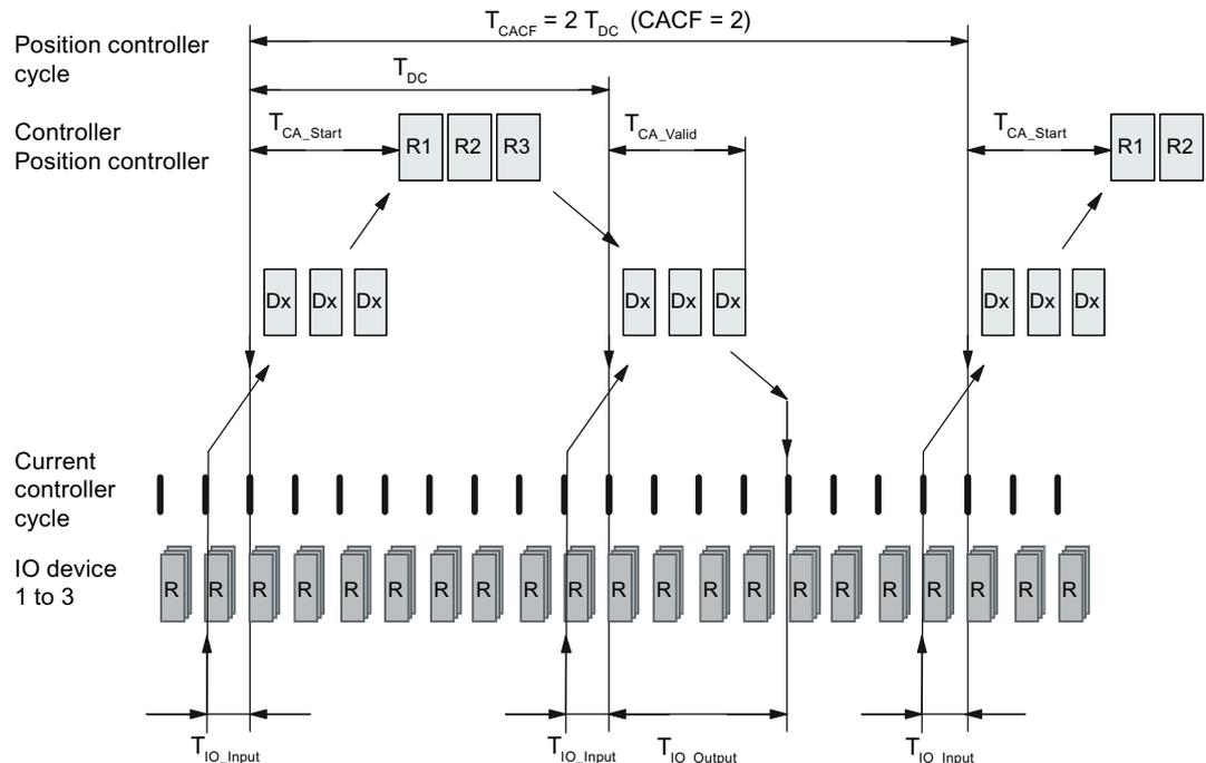
Figure 6-3 Motion Control / isochronous drive link with PROFINET, optimized cycle with CACF = 2 (Controller Application Cycle Factor)
