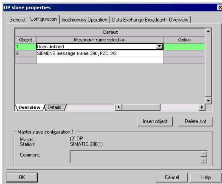
Figure 5-16 Telegram assignment for slave-to-slave communication
