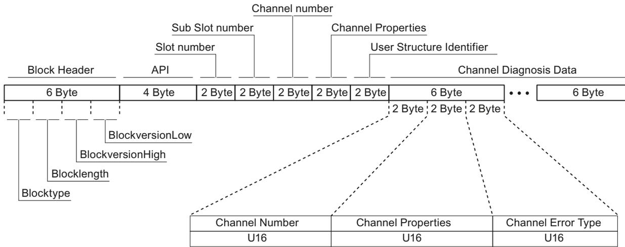
Figure 4-9 Components of a message
