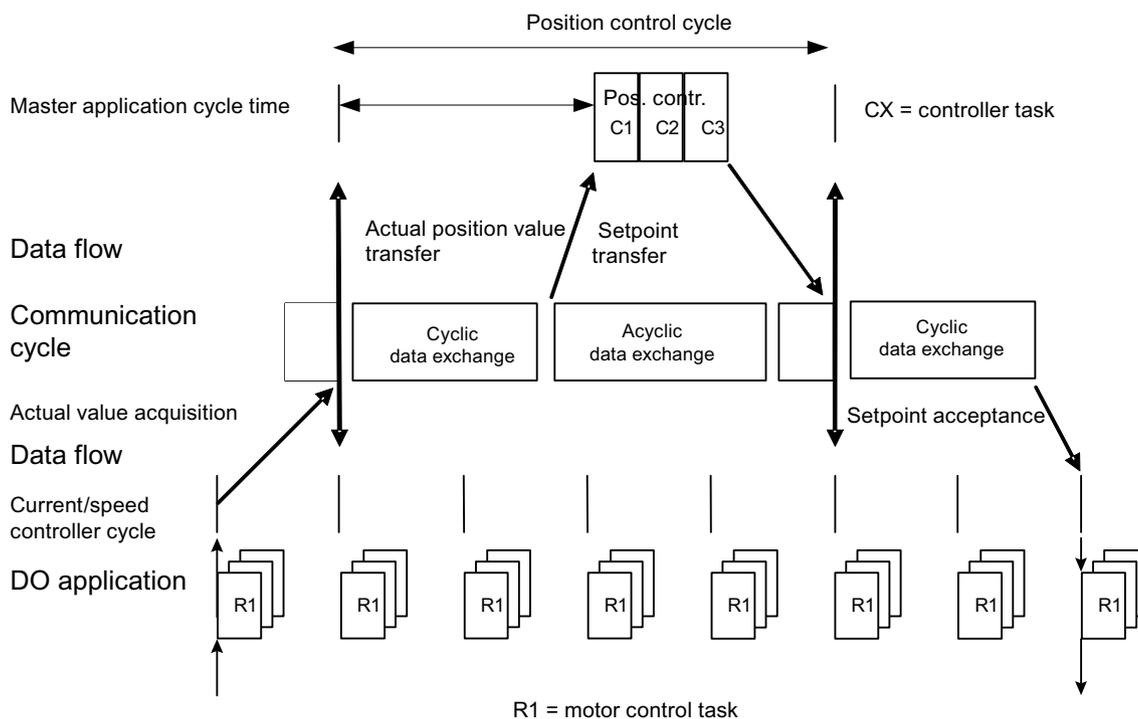
Figure 4-6 Isochronous drive coupling / motion control with PROFIdrive
