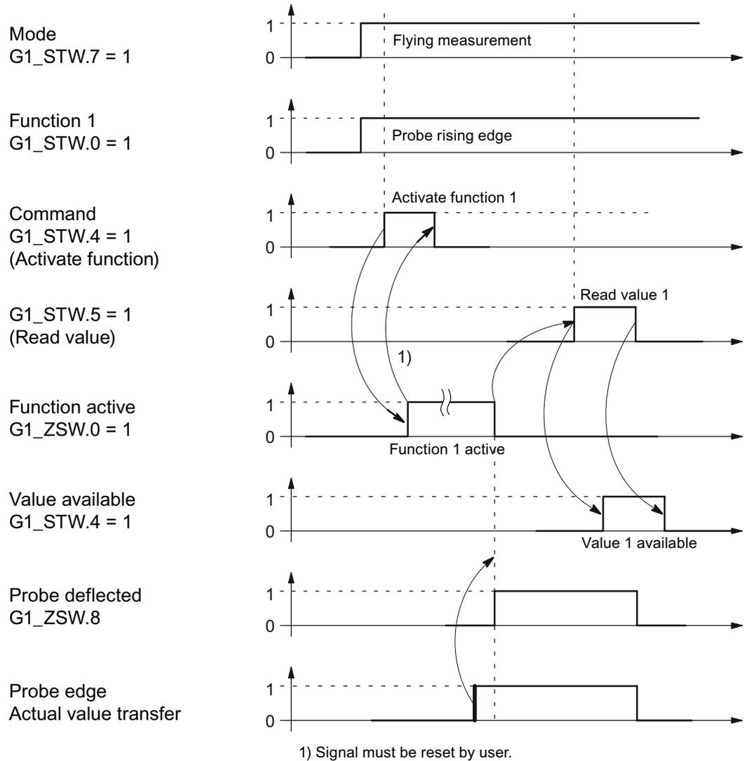
Figure 4-4 Sequence chart for "Flying measurement"
