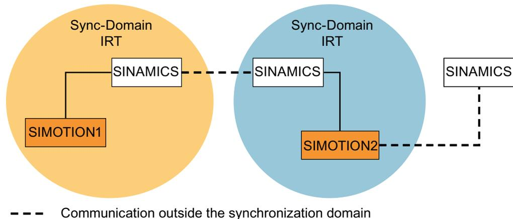
Figure 6-2 RT communication across the limits of synchronization domains
