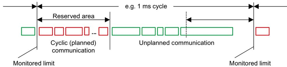
Figure 6-1 Bandwidth distribution/reservation, PROFINET IO
