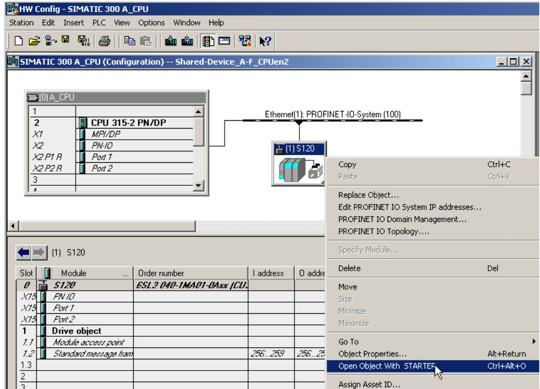
Figure 6-8 New project transferred from HW Config into STARTER
