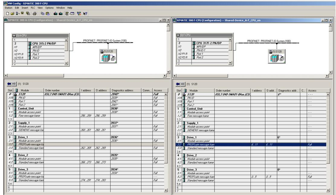
Figure 6-16 New project completed in HW Config
