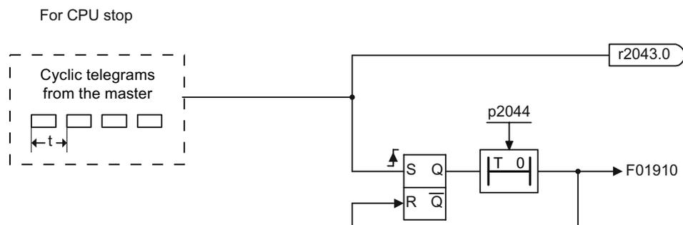
Figure 5-6 Monitoring telegram failure for a CPU stop
