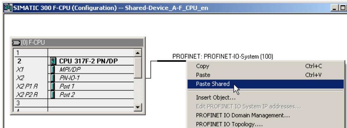
Figure 6-15 PROFIsafe controller configuration
