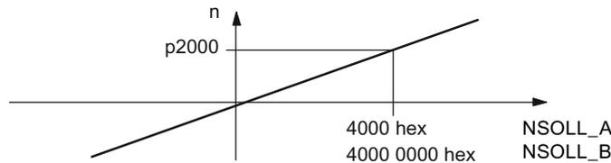
Figure 4-1 Normalization of speed
