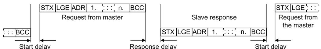
Figure 10-9 Start delay and response delay
