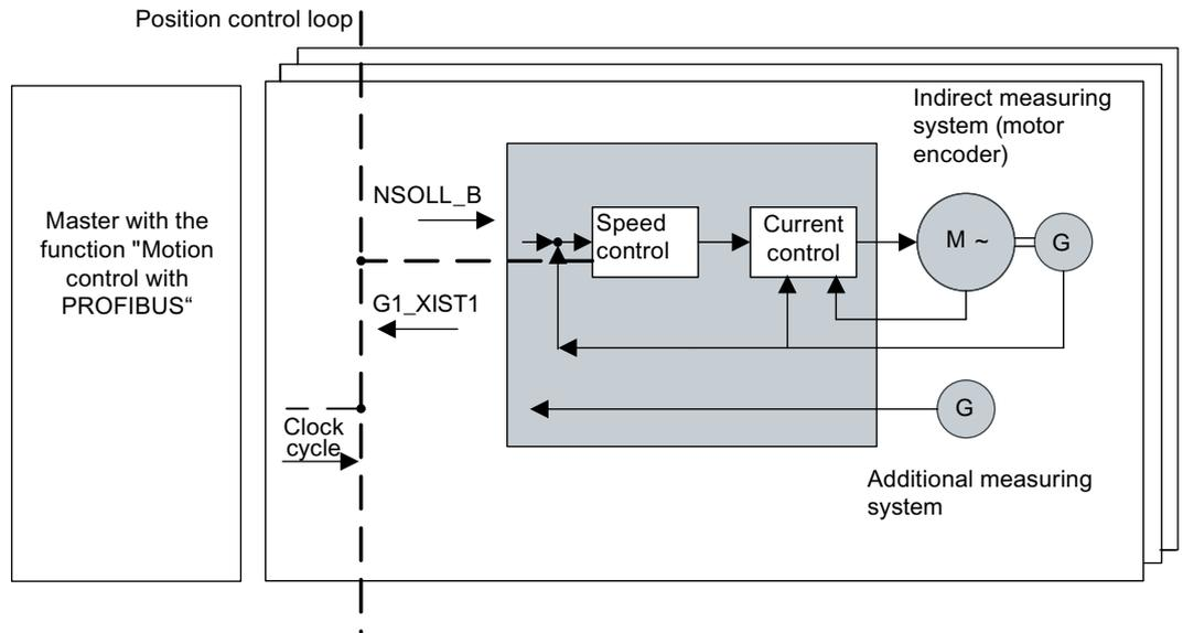
Figure 4-5 Overview of "Motion Control with PROFIBUS" (example: controller and 3 devices)
