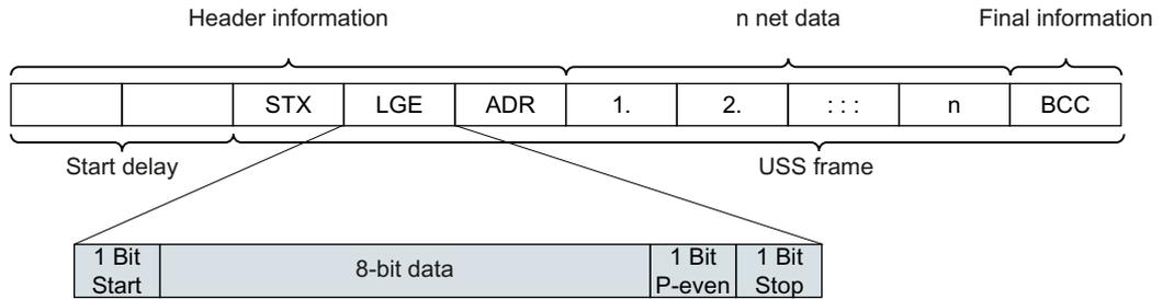
Figure 10-1 Structure of a USS telegram
