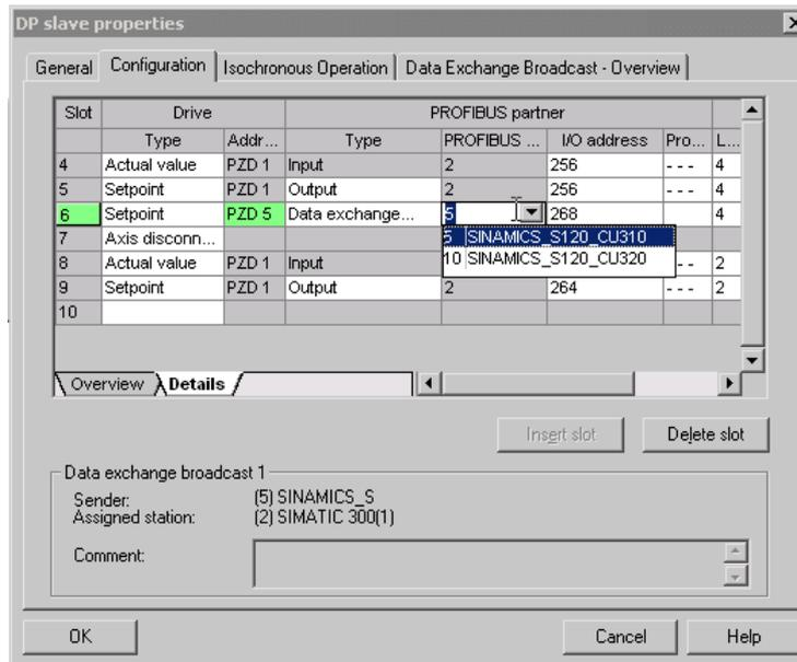
Figure 5-14 Configuring the slave-to-slave communication nodes
