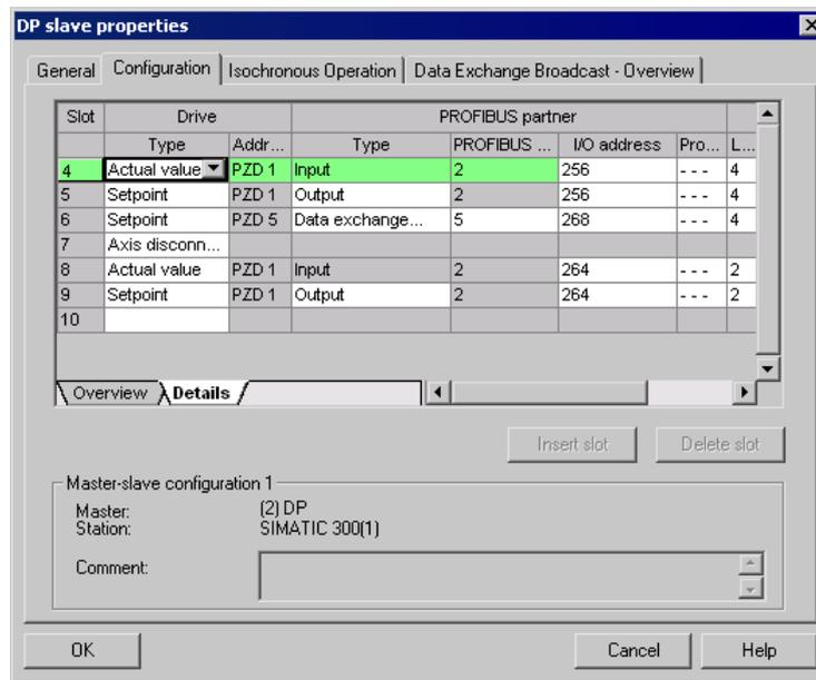
Figure 5-17 Details after the creation of the slave-to-slave communication link
