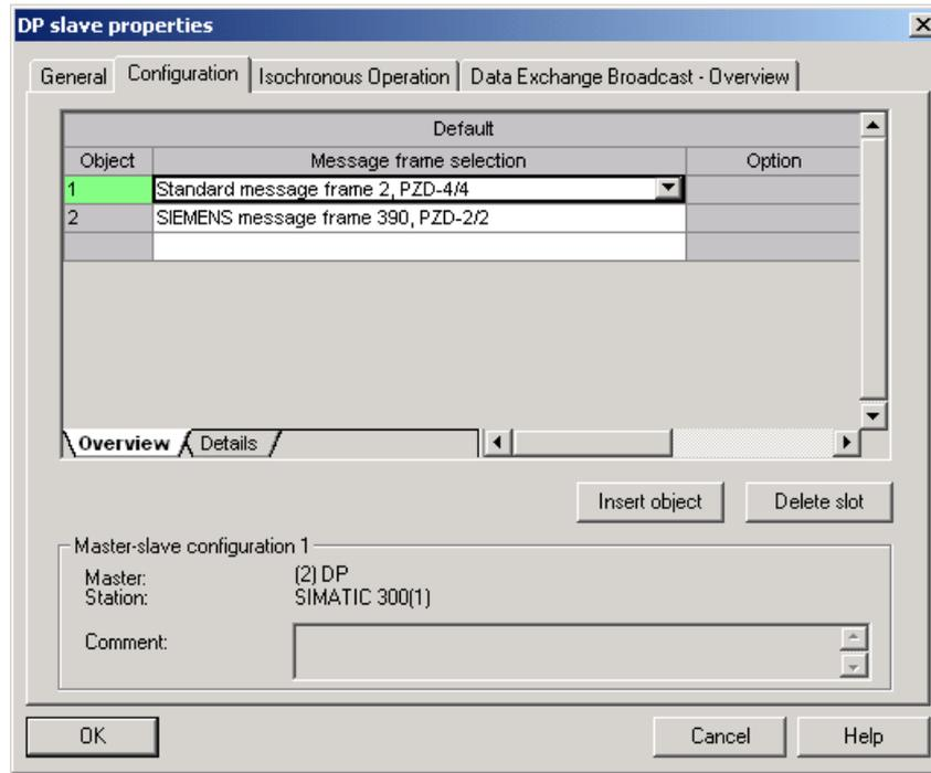
Figure 5-11 Telegram selection for drive object
