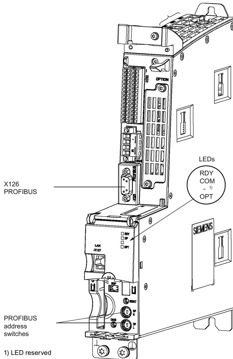
Figure 5-4 Interfaces and diagnostic LED
