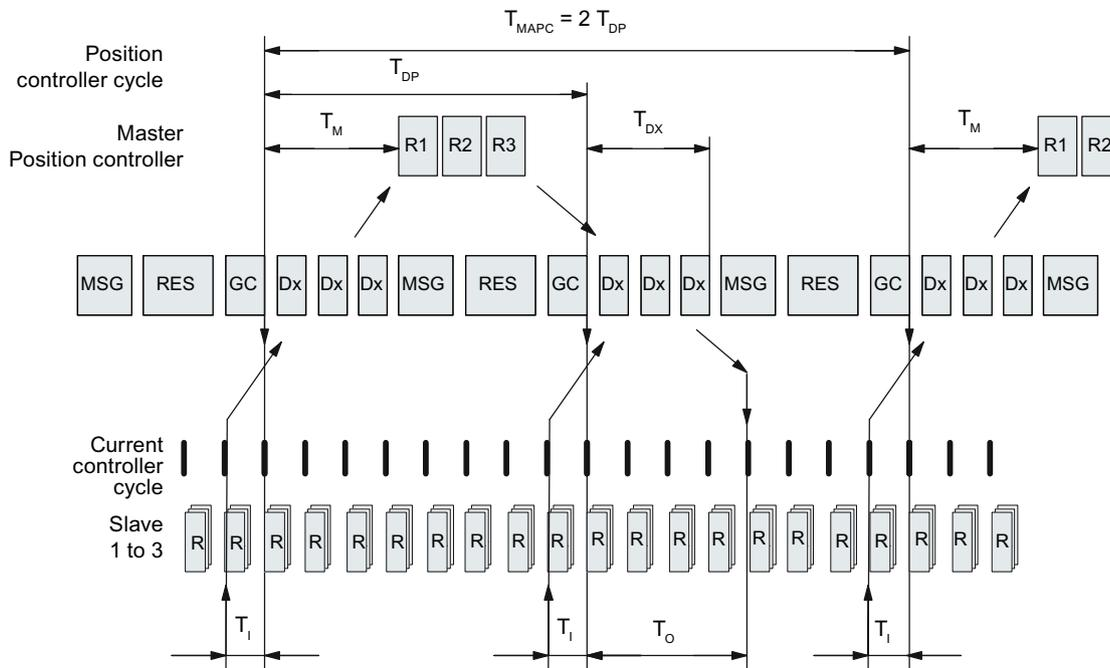
Figure 5-7 Motion control / isochronous drive coupling with PROFIBUS, optimized cycle with  $T_{MAPC} = 2 \cdot T_{DP}$
