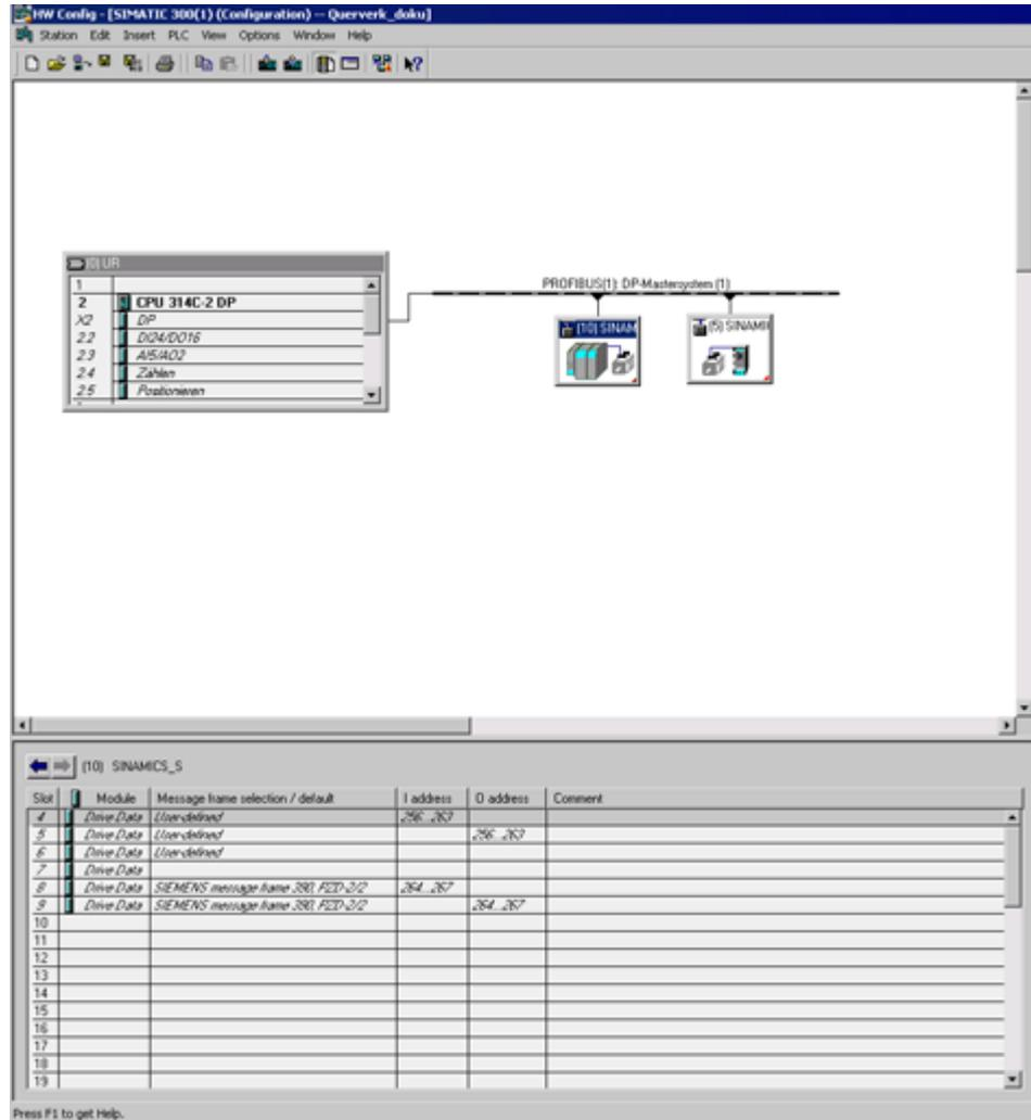
Figure 5-10 Example project of a PROFIBUS network in HW Config
