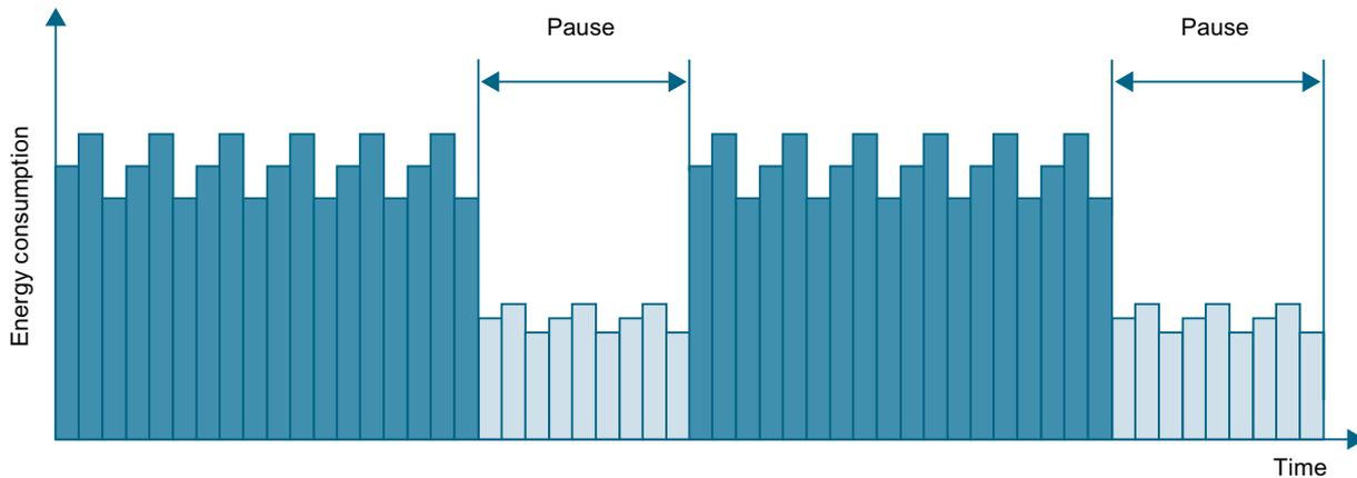
Figure 6-20 Energy saving during pauses with PROFIenergy
