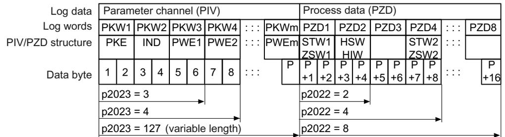
Figure 10-2 USS telegram - user data structure
