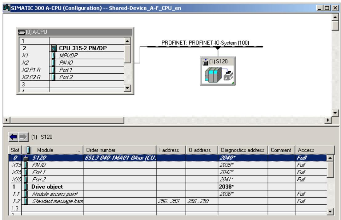
Figure 6-7 Automation controller created in HW Config
