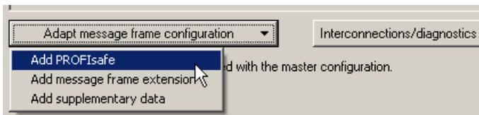
Figure 6-10 Add the PROFIsafe telegram to the drive
