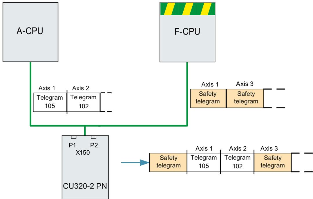
Figure 6-5 Example, communication sequence
