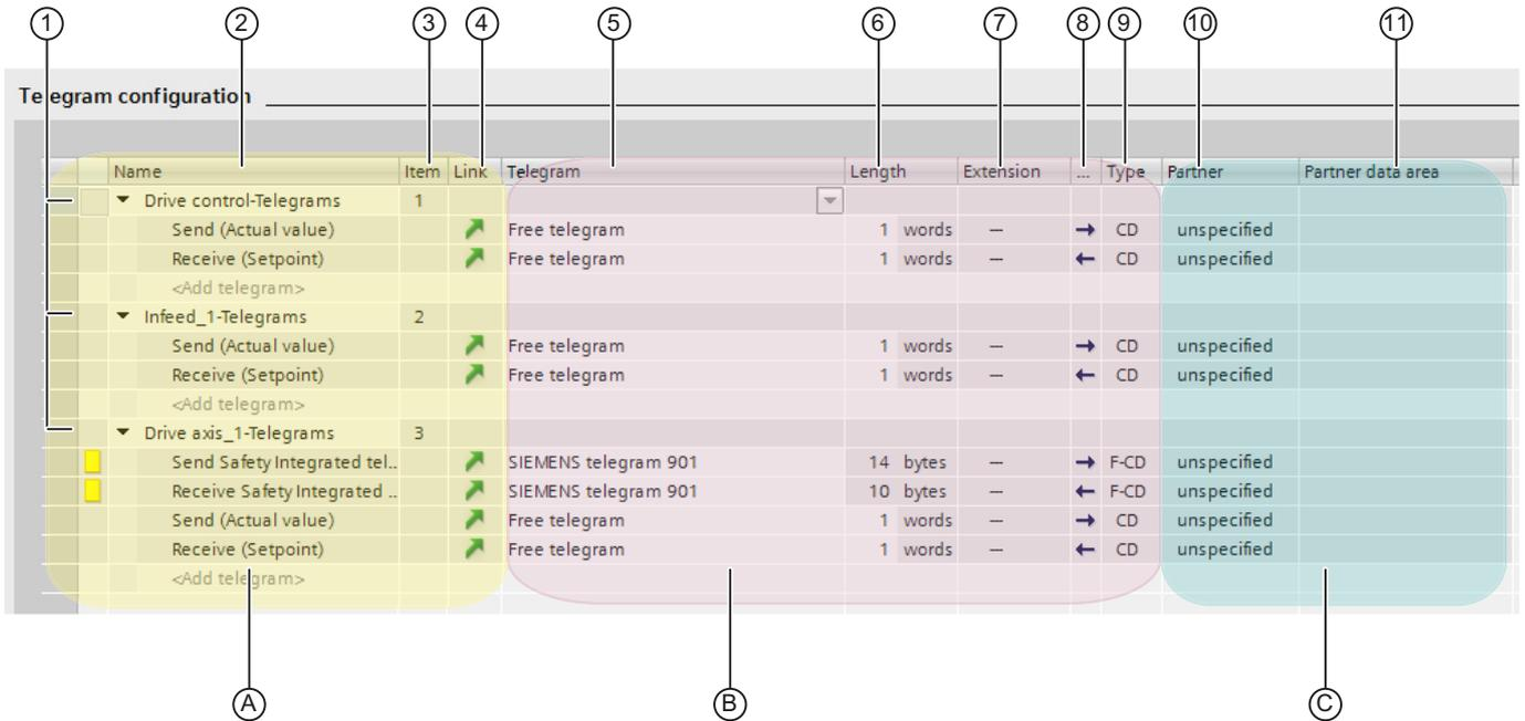
Figure 4-10 Example: Telegram configuration with several drive objects
