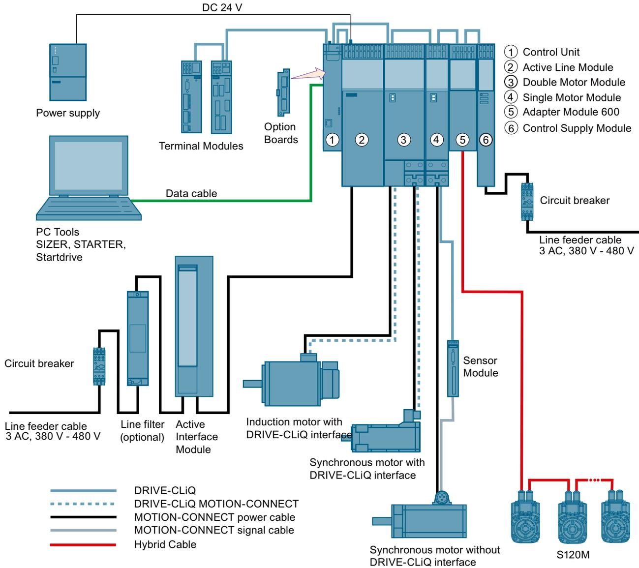
Figure 3-3 System overview, SINAMICS S120 with distributed servo drive technology S120M
