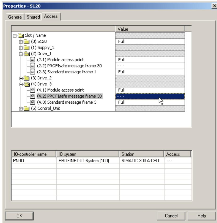
Figure 6-14 Safety telegrams of the A-CPU enabled
