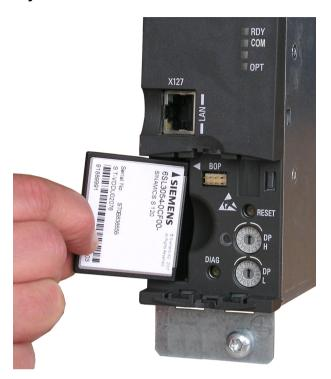
Figure 4-20 Slot for the memory card
